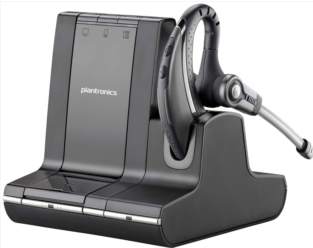
Figure 1: The Plantronics Savi Office W730 headset docked in its base station. The base station serves as a charging dock and connectivity hub for PC, desk phone, and mobile devices.
