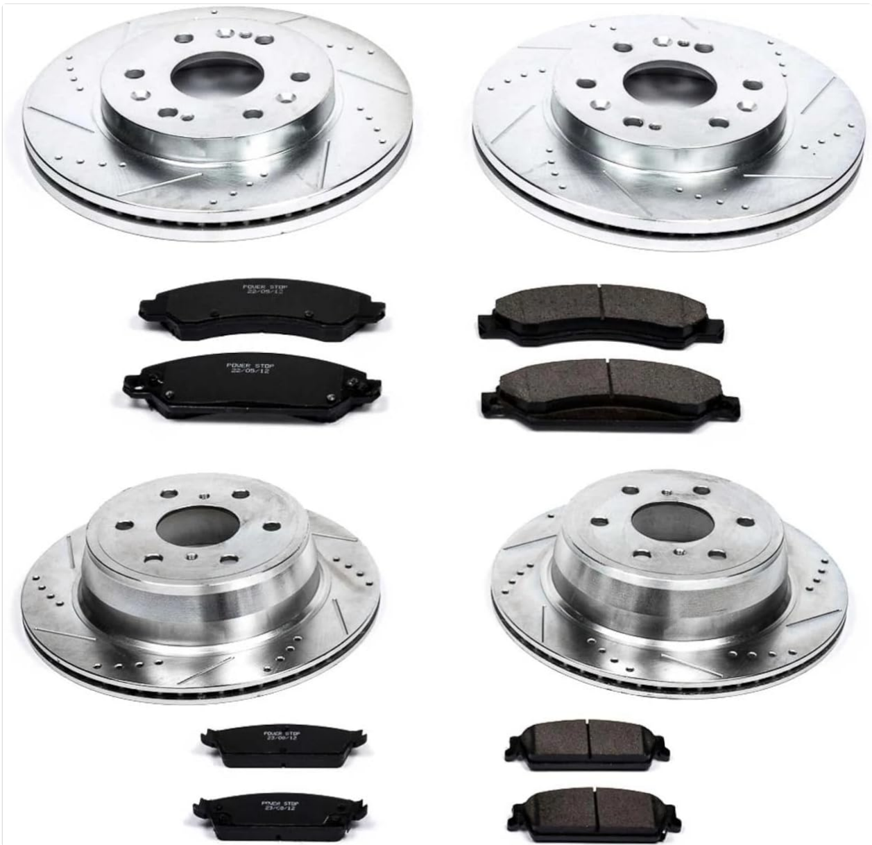
Figure 2: Contents of the Power Stop K2068 Brake Kit.
