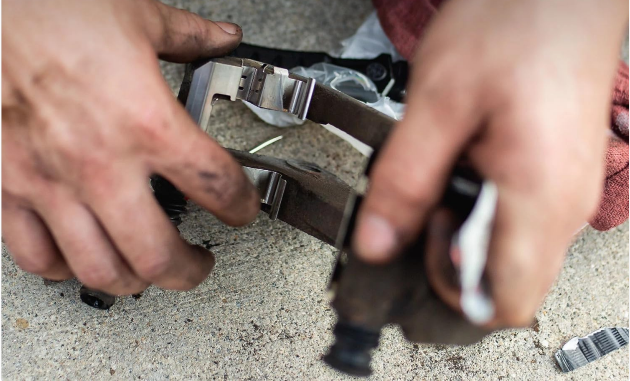
Figure 6: Rounded slots for debris removal.
