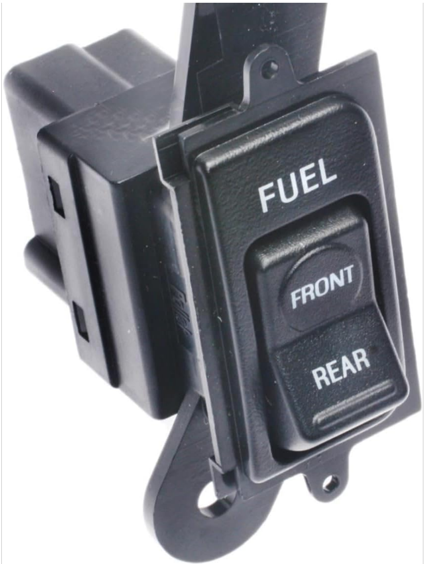
Figure 1: Front view of the DS-2268 Switch, showing the 'FUEL', 'FRONT', and 'REAR' labels. This image illustrates the primary user interface of the switch.
