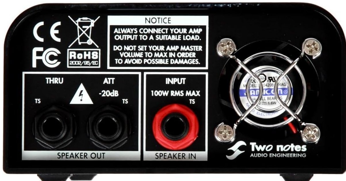
Figure 3.2: Rear Panel Connections. This image displays the rear panel of the Torpedo Captor 4, featuring the 'SPEAKER IN' (100W RMS MAX TS) and 'SPEAKER OUT' (THRU and ATT -20dB TS) jacks. A prominent notice warns users to always connect their amp output to a suitable load and not to set the amp master volume to max. A cooling fan is also visible.
