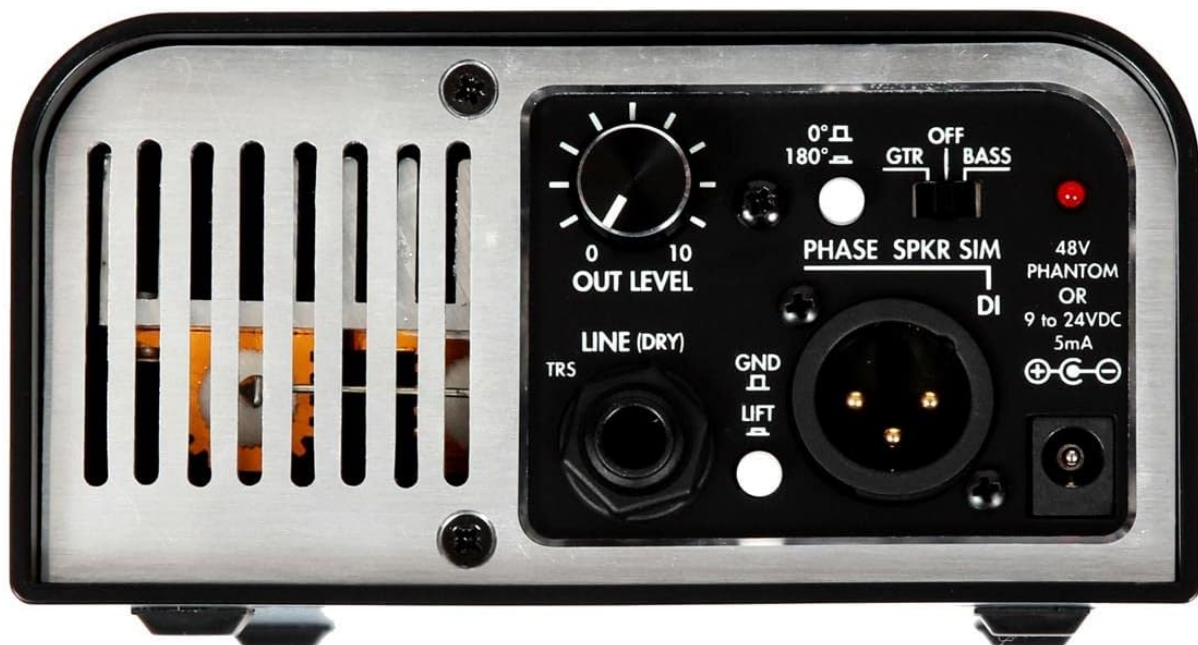
Figure 3.3: Front Panel Controls and DI Output. This image shows the front panel of the Torpedo Captor 4, highlighting the 'LINE (DRY)' TRS output, 'DI' XLR output with 'GND LIFT' switch, 'OUT LEVEL' knob, 'PHASE' switch (0°/180°), and 'SPKR SIM' switch (OFF/GTR/BASS). A 48V Phantom Power indicator and a DC input for 9 to 24VDC are also visible.
