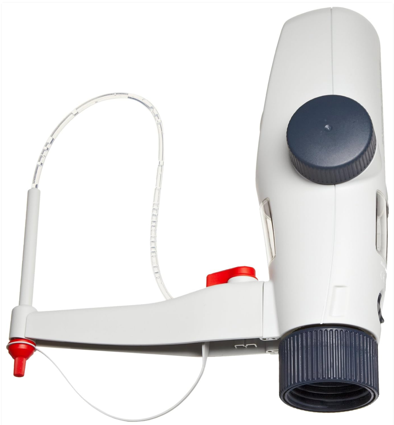
Figure 2: Side view of the Titrette Bottletop Burette, highlighting the compact design and the titration tube's adjustability.
