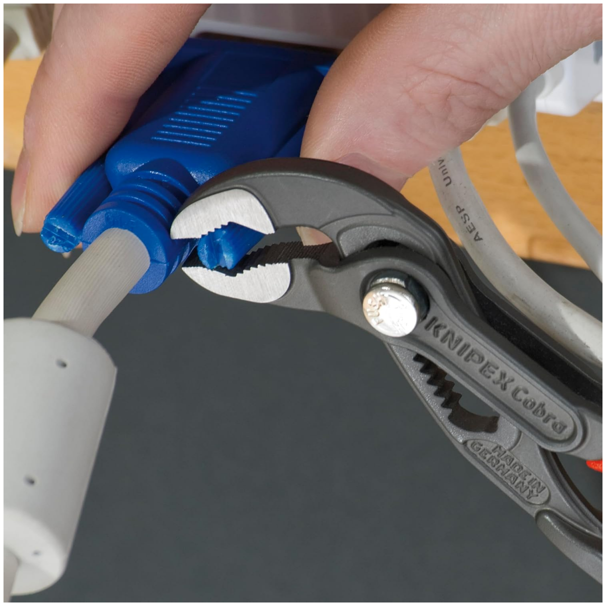
Figure 5: The pliers gripping a larger cable connector, showcasing their adaptability to various sizes and shapes.
