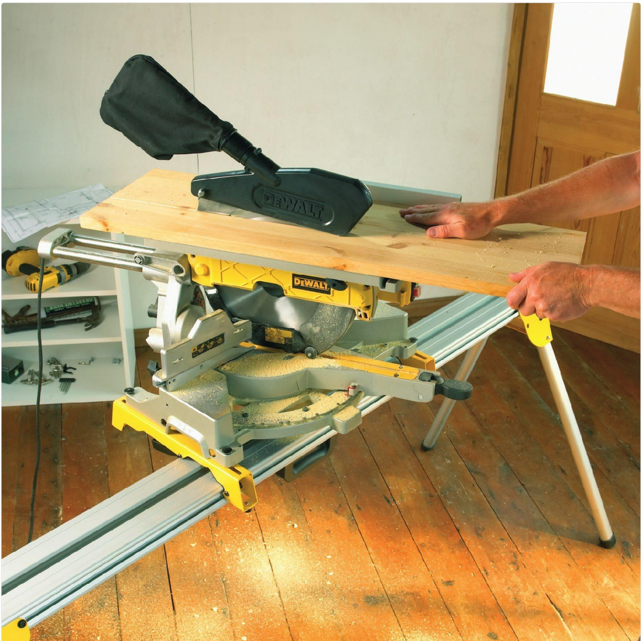
Figure 2: Ripping operation using the upper table of the DEWALT D27112-QS.
