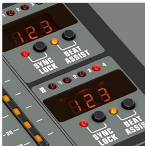
Figure 4: Close-up of the dual auto-BPM counter, showing the digital display and sync indicators for precise beat matching.
