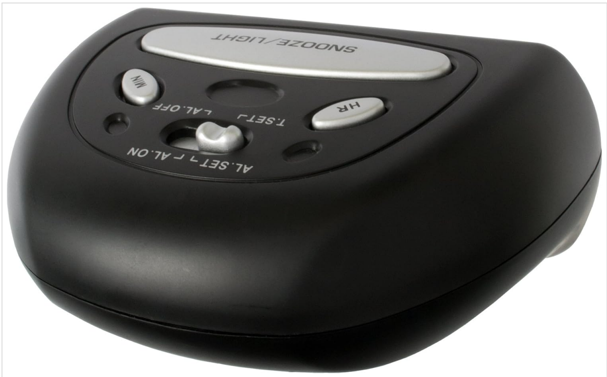
Figure 2: Top view of the alarm clock, highlighting the control buttons. These include buttons for setting hours (HR) and minutes (MIN), time setting (T.SET), alarm setting (AL.SET), and a switch for alarm on/off (AL.ON/OFF). The large button at the top is for SNOOZE/LIGHT.
