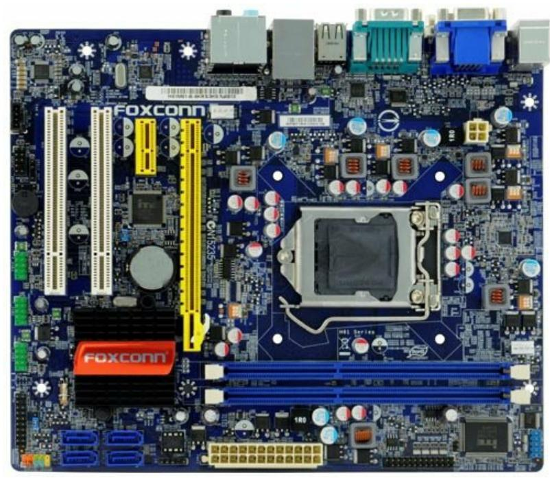
This image displays the Foxconn H61MX motherboard, showcasing its various components such as the CPU socket, memory slots, expansion slots, and I/O ports. This visual aid helps in identifying the locations for component installation.
