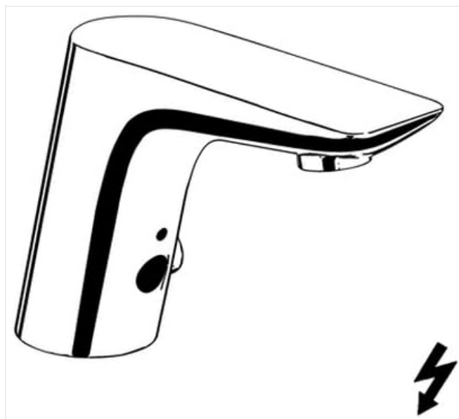
Figure 3.2: Line drawing illustrating the general form and key features of the KLUDI BALANCE Faucet. This diagram provides a simplified view, emphasizing the sensor location and the overall profile of the unit.
