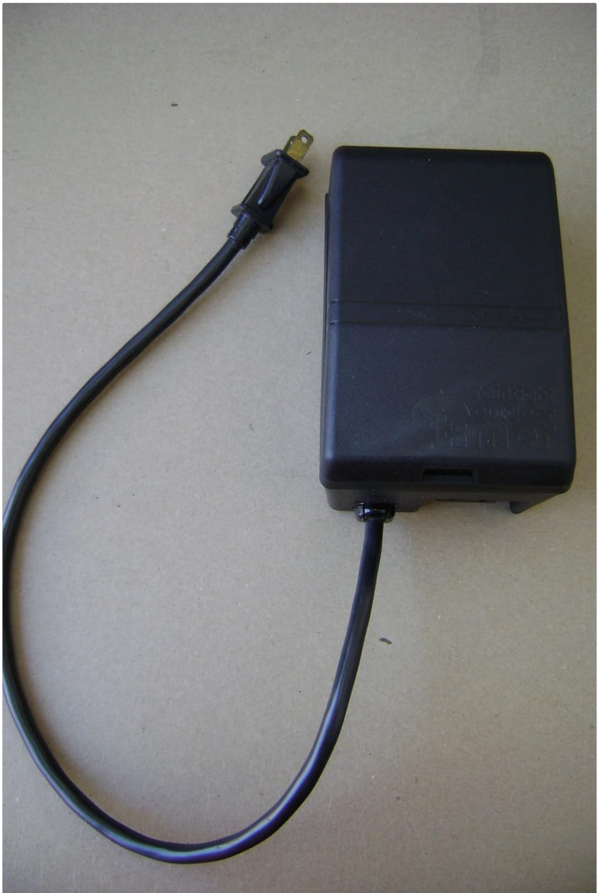
Figure 2: The Intermatic HB32R outdoor timer in its closed position, showcasing its compact, raintight black casing. The attached power cord with a two-prong plug extends from the unit.
