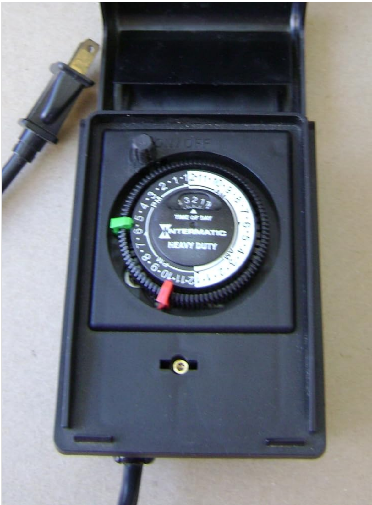
Figure 1: Front view of the Intermatic HB32R timer with the protective cover open, revealing the central 24-hour programming dial. The dial features markings for time and slots for inserting red (ON) and green (OFF) pins. A black power cord with a two-prong plug is visible on the left.
