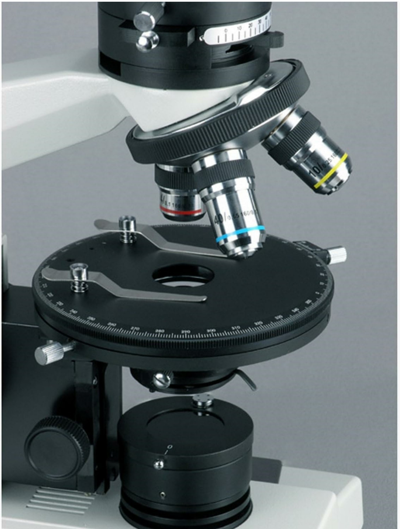
Figure 3: Close-up view of the objective lenses mounted on the nosepiece and the round graduated stage, highlighting the precision components.
