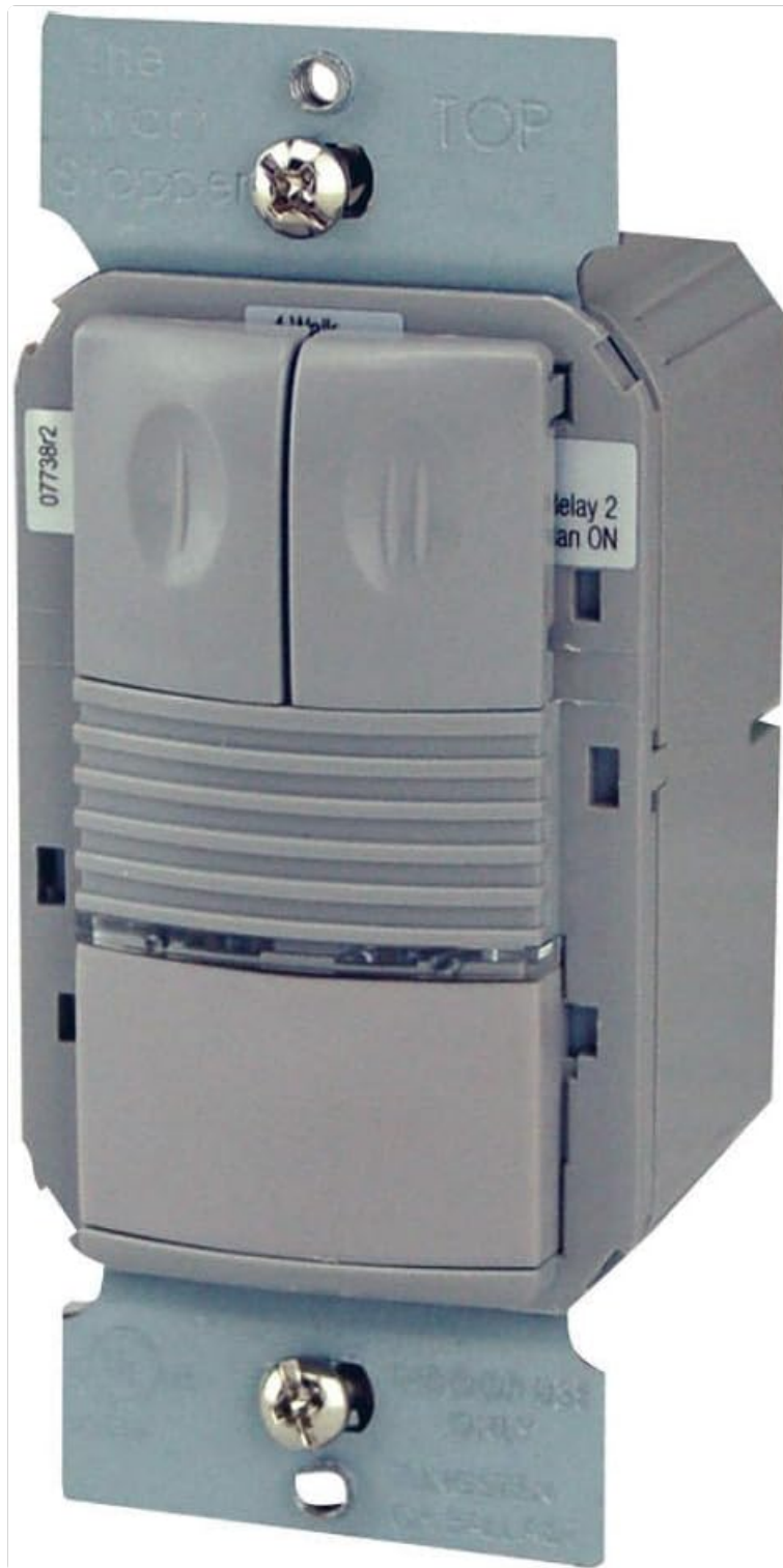
Figure 1: Front view of the Wattstopper PW-200-G Occupancy Sensor. The sensor is grey, designed for wall mounting, and features two push buttons at the top for manual control of the dual relays. The lower section contains the PIR lens for motion detection. Mounting screws are visible at the top and bottom of the metal bracket.
