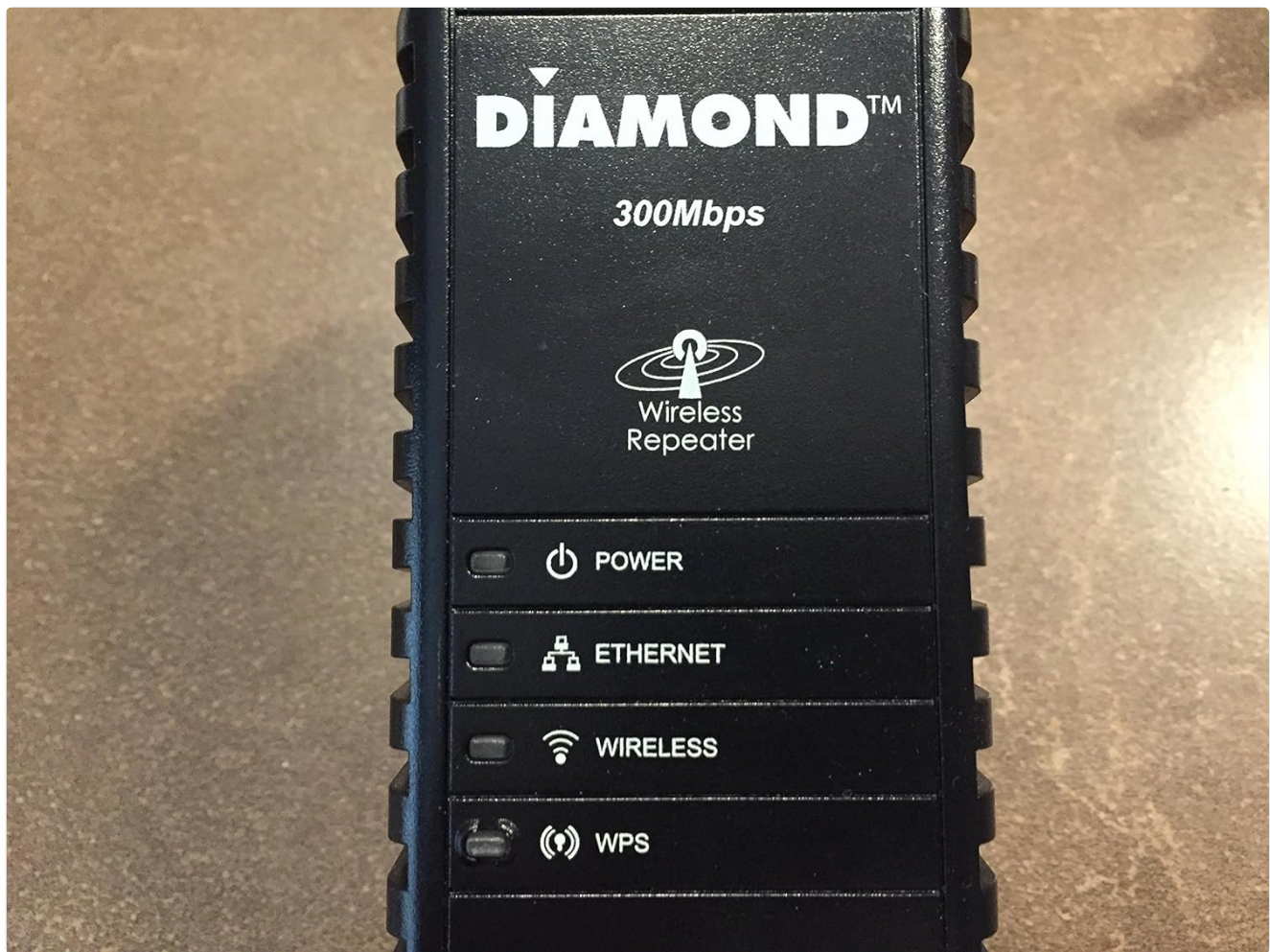
Image: A close-up view of the WR300N's front panel, showing the "DIAMOND 300Mbps Wireless Repeater" branding and four LED indicators.
