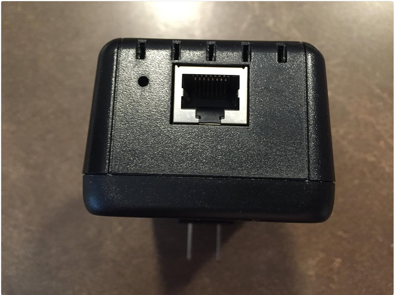
Image: The top view of the WR300N, highlighting the Ethernet port and a small reset button hole.
