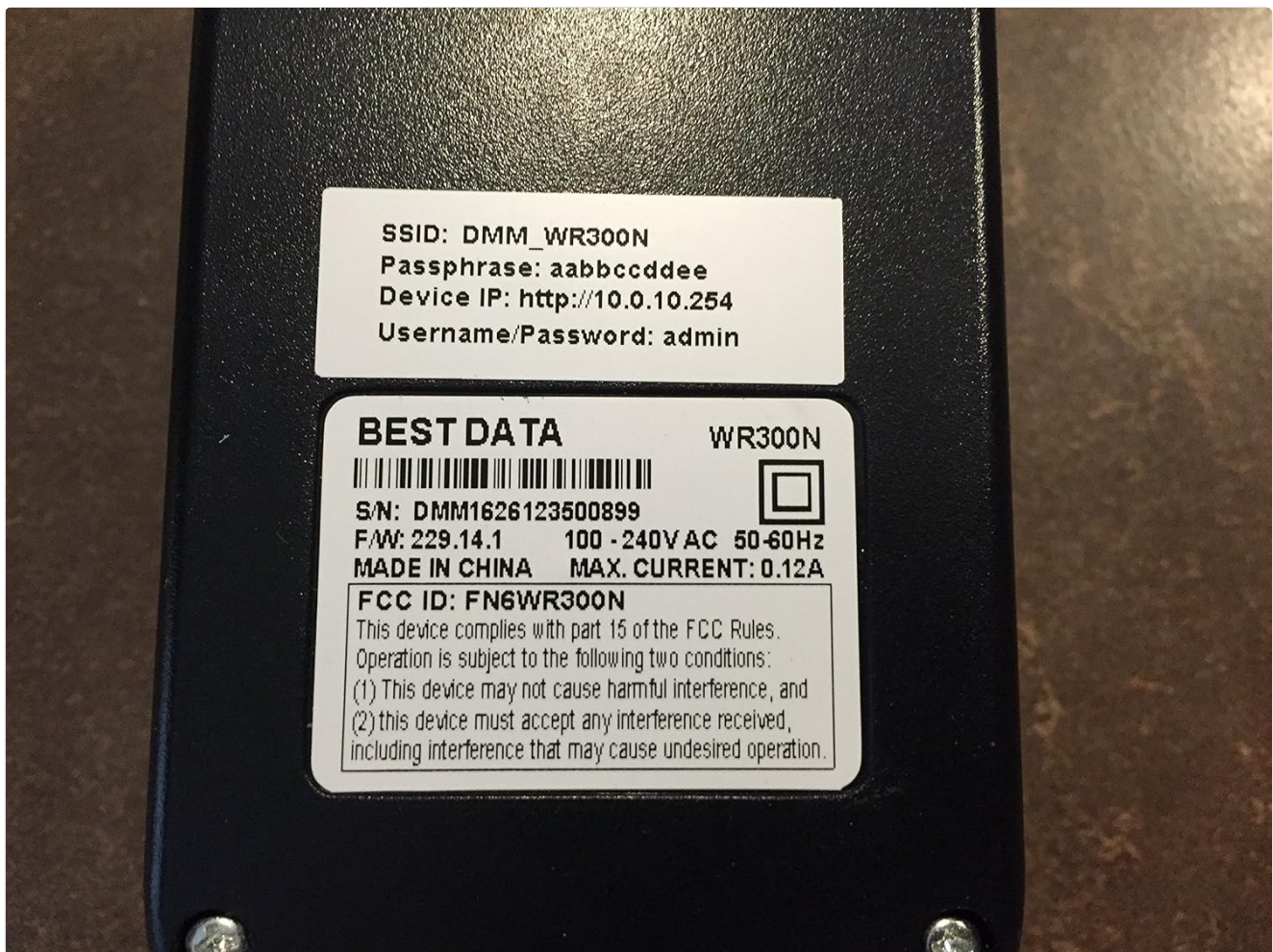
Image: A close-up of the product label on the back of the WR300N, showing default network information.
