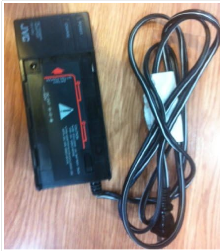
Image: The JVC AC power adapter, used for charging the camcorder's battery and powering the unit directly from a wall outlet.
