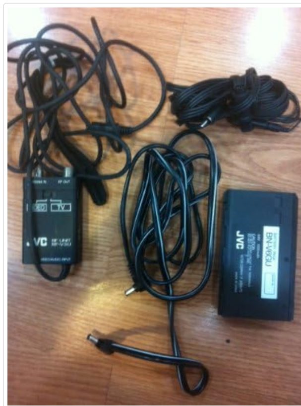
Image: Various camcorder accessories including the JVC RF unit, a rechargeable battery pack (BN-V60U), and several connecting cables for audio/video output.
