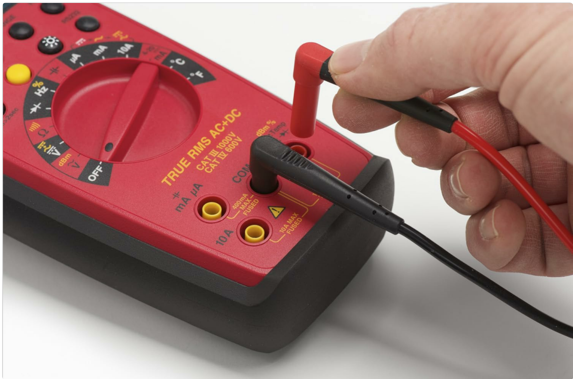
Figure 2: Fluke TL175 Test Leads properly connected to a digital multimeter.
