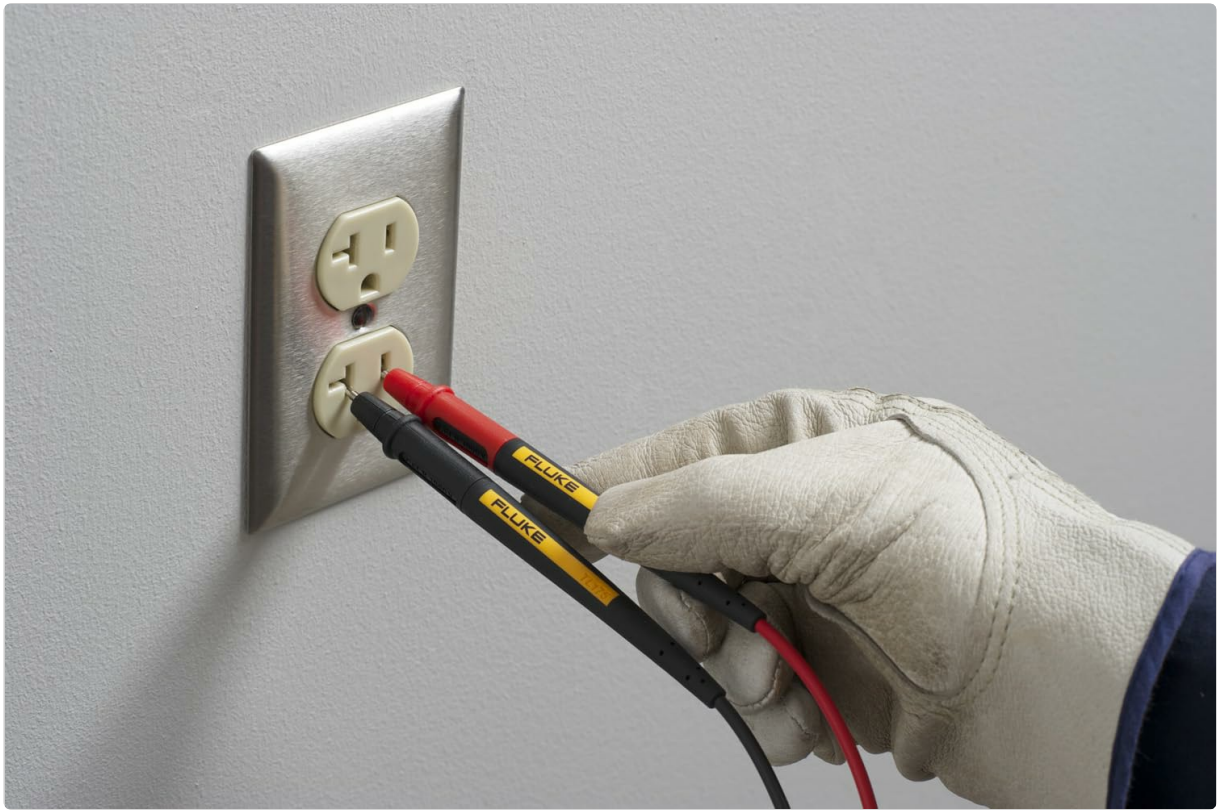
Figure 5: Fluke TL175 Test Leads used to test an electrical outlet, suitable for CAT II applications with tips fully exposed.
