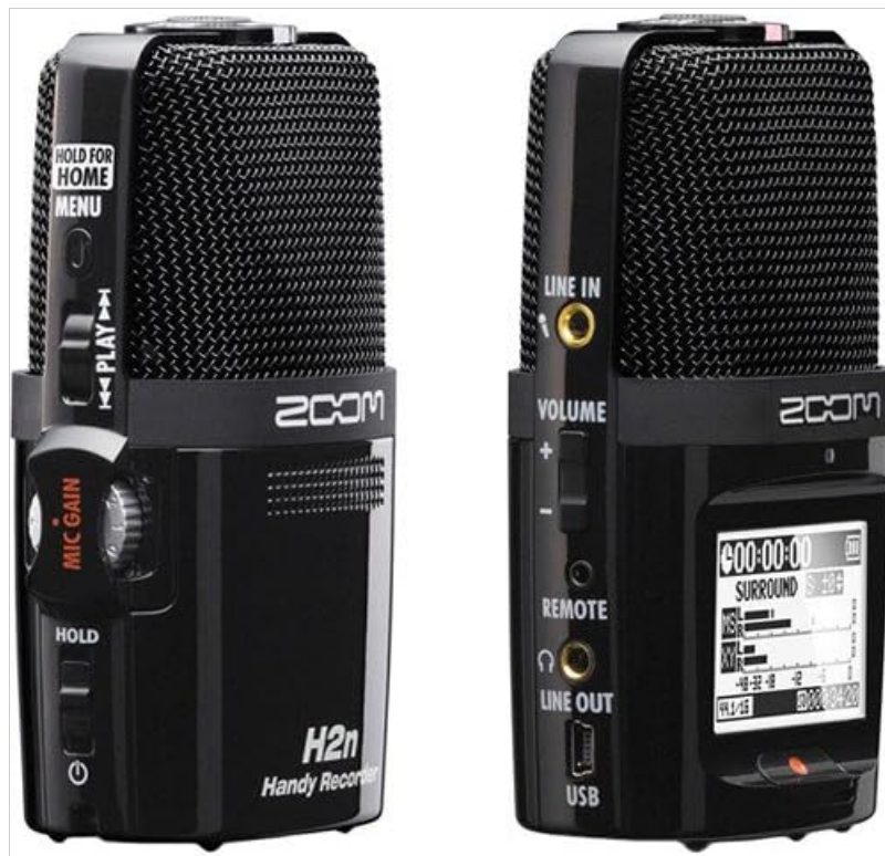
Figure 2.2: Side views illustrating the various controls and input/output ports, including Line In, Line Out, USB, Volume, and Mic Gain.
