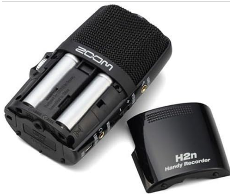
Figure 3.1: Battery compartment of the Zoom H2n, open to show the insertion of two AA batteries.
