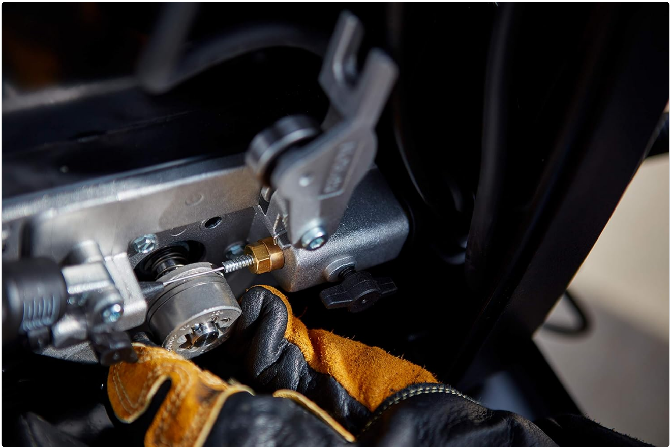
Image 4.1: Detailed view of the wire feed mechanism, showing the drive roll and wire path for proper installation.
