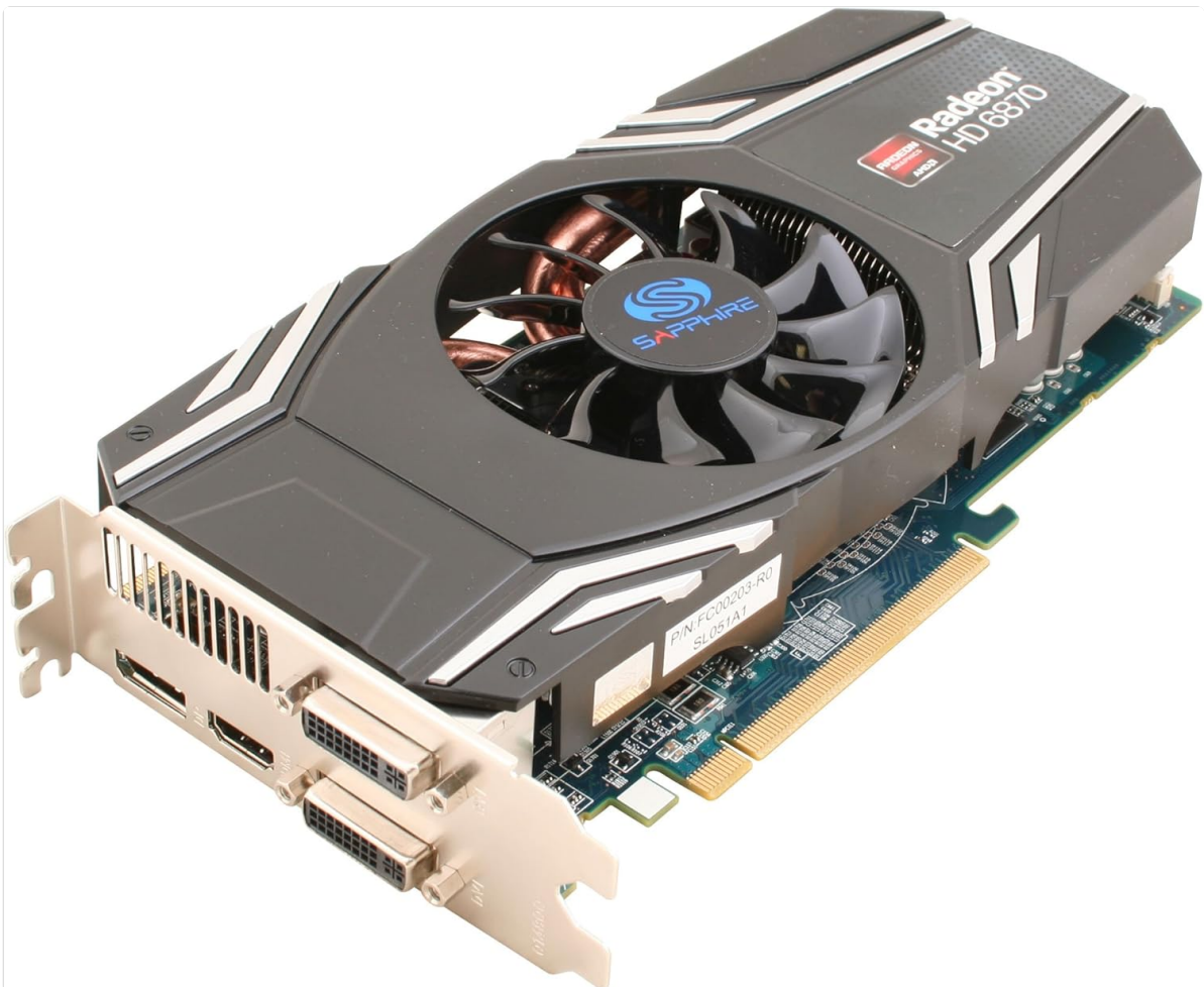
Figure 4.1: Graphics Card PCI Express Connector
