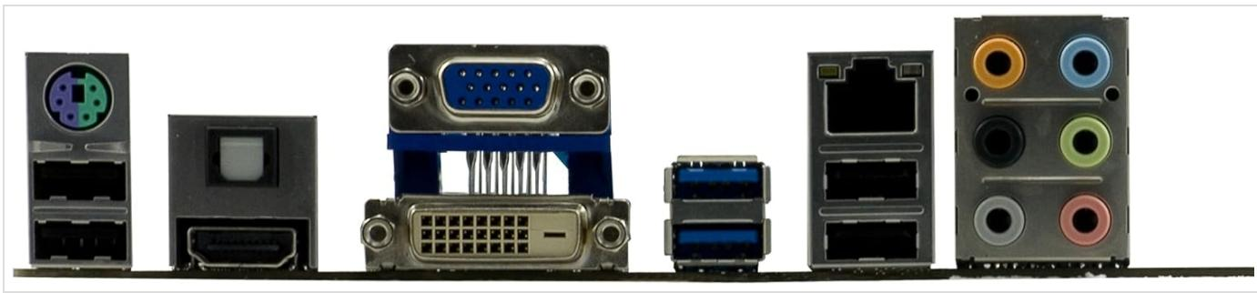
The rear I/O panel of the ASUS P8Z68-V LE motherboard includes a PS/2 port, USB 2.0 ports, USB 3.0 ports, HDMI, DVI, VGA, Gigabit Ethernet, and 8-channel audio jacks, providing comprehensive connectivity options.
