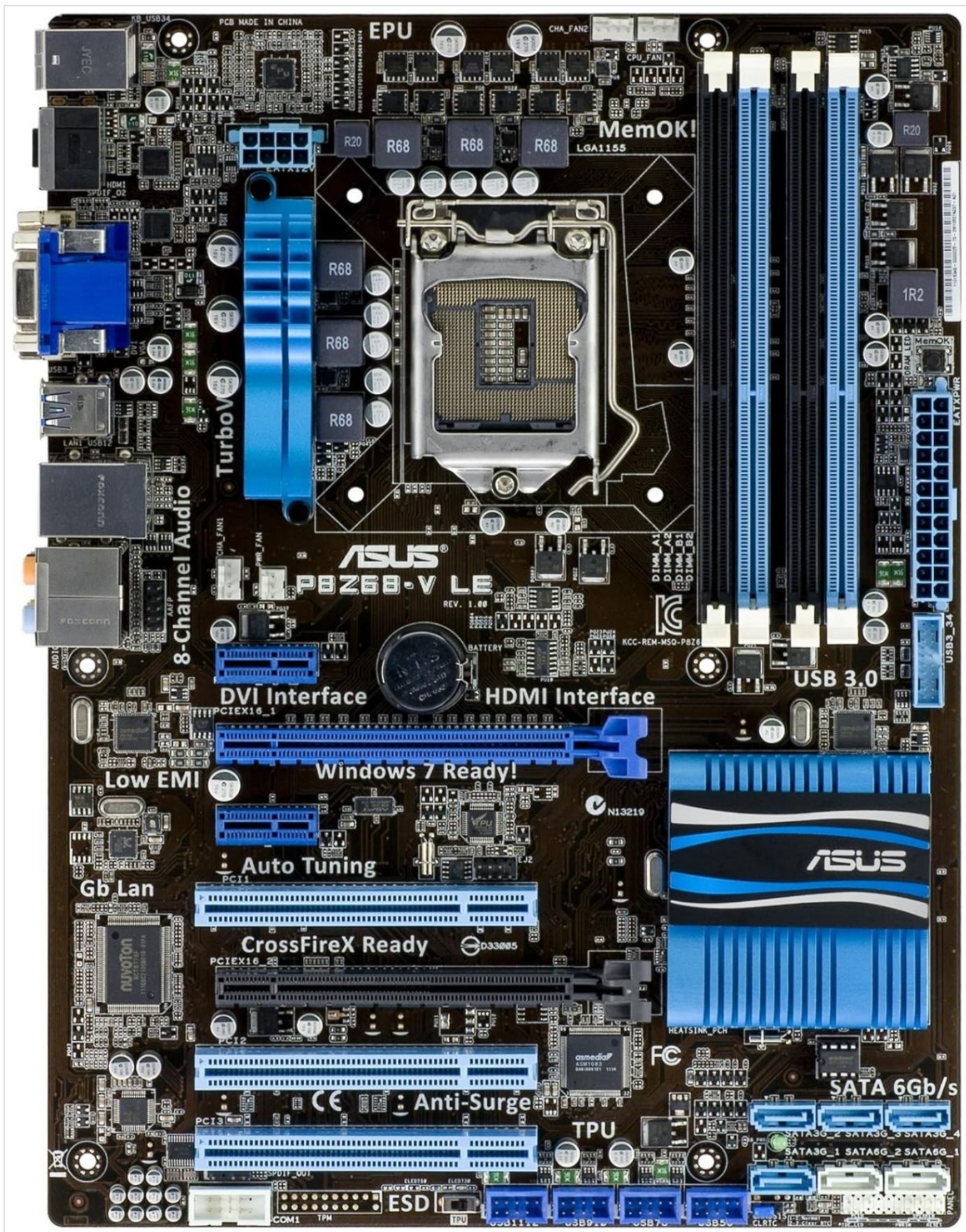
This image displays the full layout of the ASUS P8Z68-V LE motherboard, highlighting key components such as the LGA 1155 CPU socket, four DDR3 DIMM slots, multiple PCIe expansion slots, SATA ports, and various headers for front panel connections.
