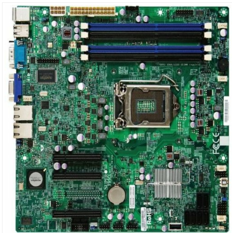
Figure 1: Supermicro X9SCL-B Server Motherboard. This image displays the overall layout of the motherboard, including the CPU
