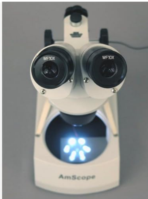
Figure 4: Top-down view showing the stage plate and the active lower LED illumination.
