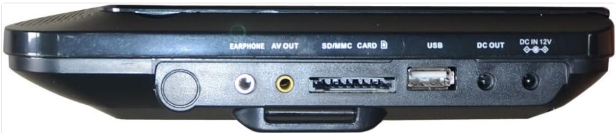
Image 2.1: Rear view of the main DVD player unit, highlighting the various input/output ports including earphone, AV out, DC in 12V, and DC out.
