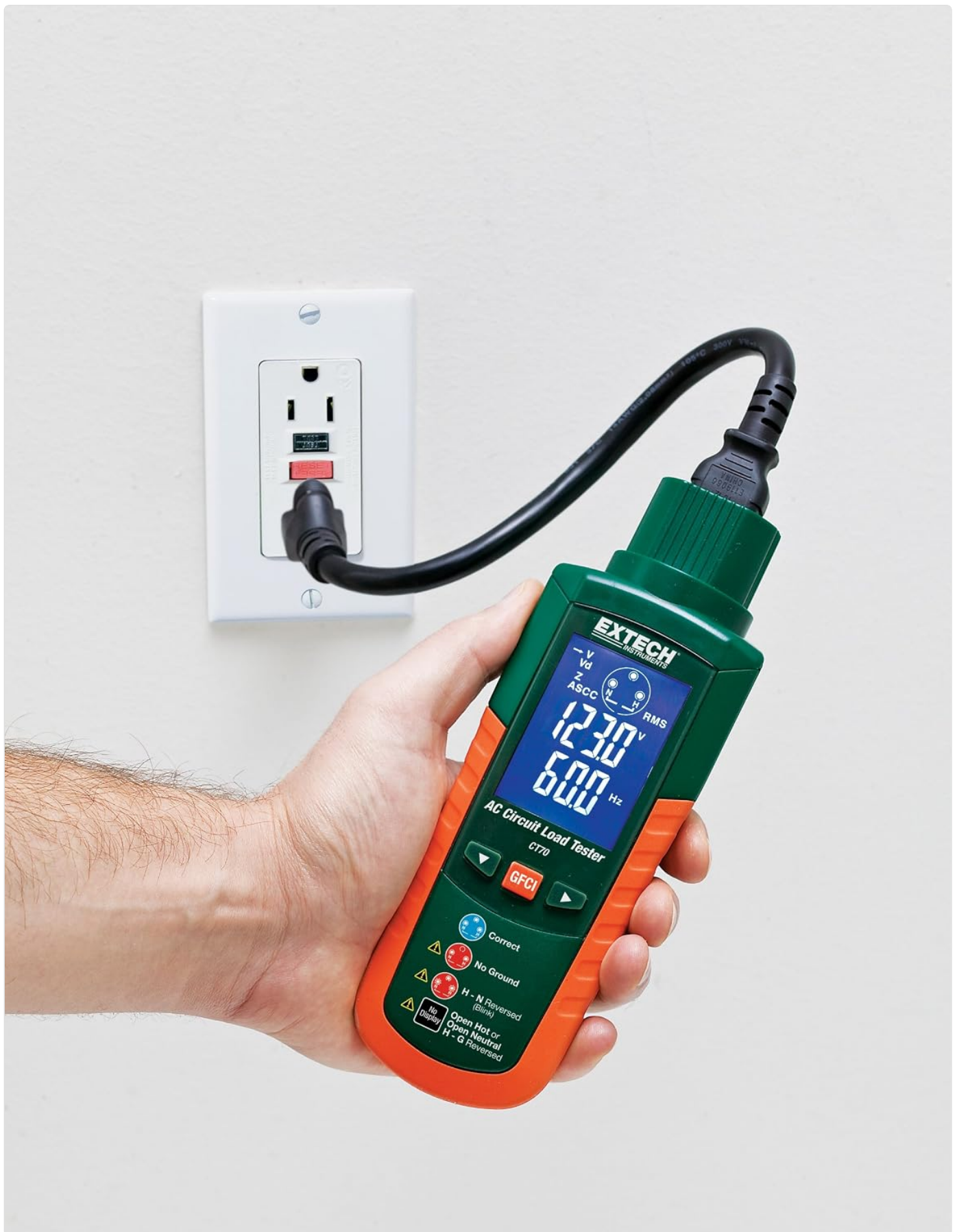
Figure 4.3: Testing a GFCI outlet with the Extech CT70.
