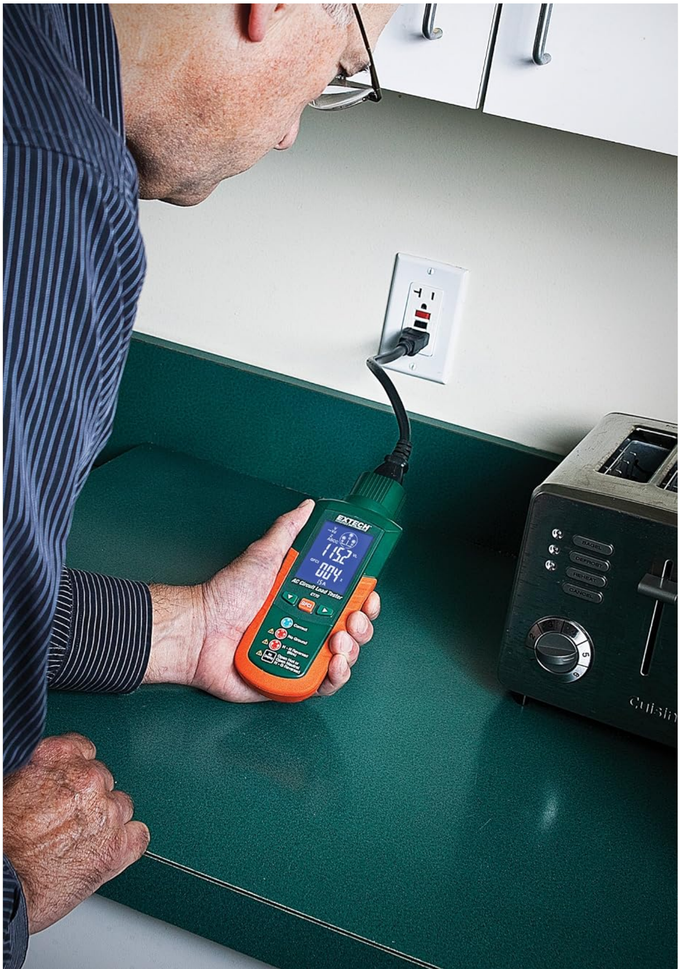
Figure 4.1: The Extech CT70 in use, displaying voltage and wiring status.
