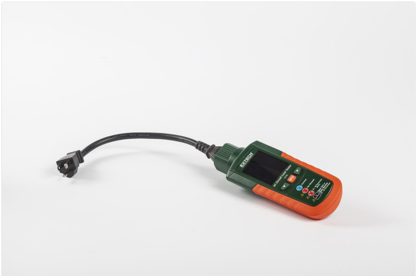
Figure 3.1: The Extech CT70 with its AC test cord, ready for connection.
