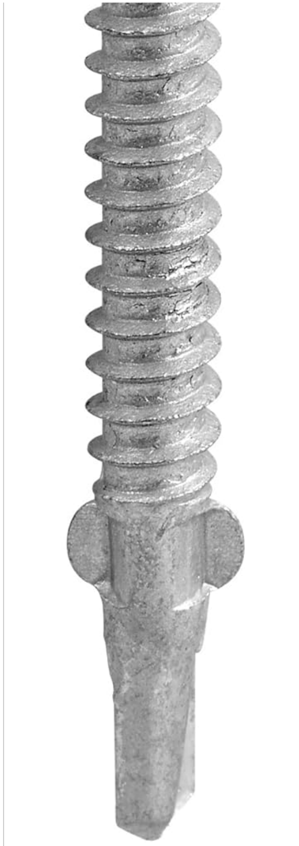
Figure 1: A single TIMco LW50B self-drilling screw. The image displays the hex head, threaded body, wing tips, and the self-drilling point. The screw has a bright zinc plated finish.
