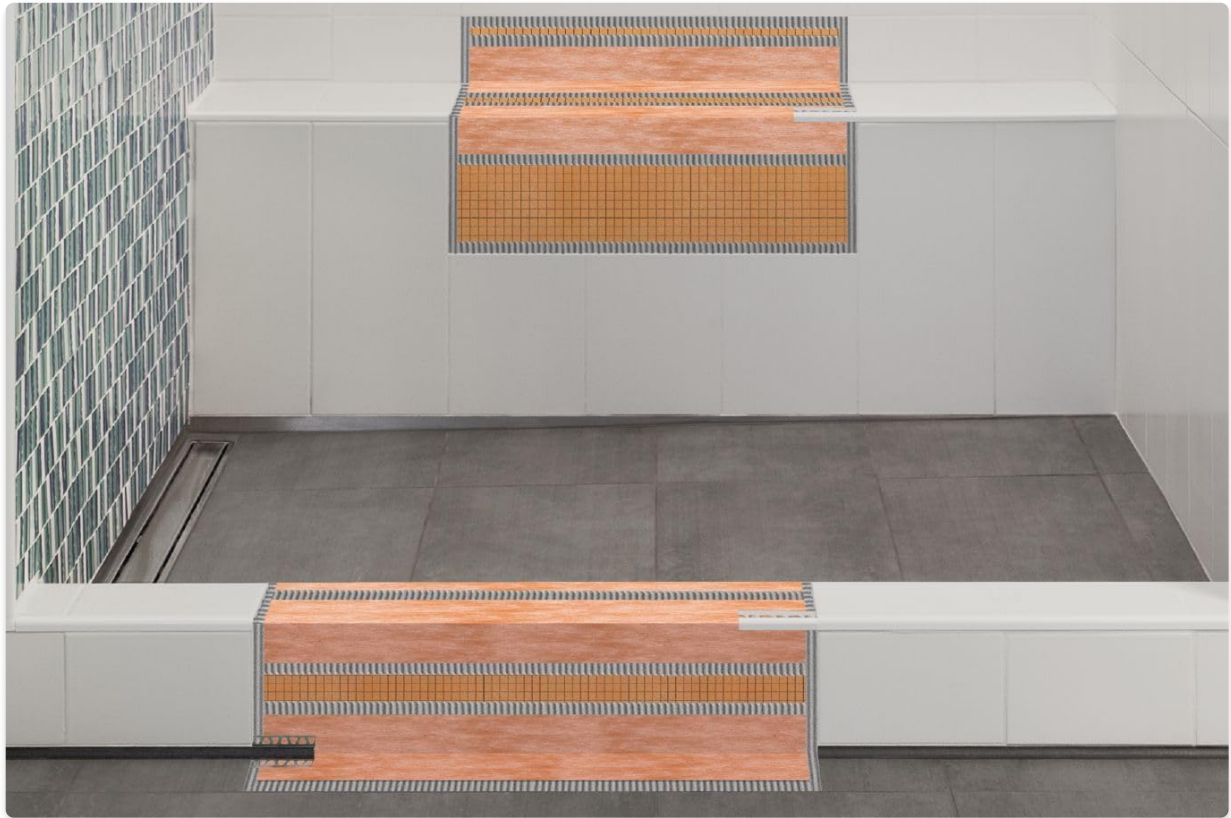
Image 3.1: A diagram illustrating the strategic placement of Kerdi Band in a shower corner to ensure a waterproof seal.
