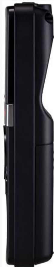
Image 2: Side view of the Olympus VN-7200 Digital Voice Recorder. This view shows the POWER/HOLD slide switch located on the left side of the device, used to turn the recorder on/off or lock its controls.
