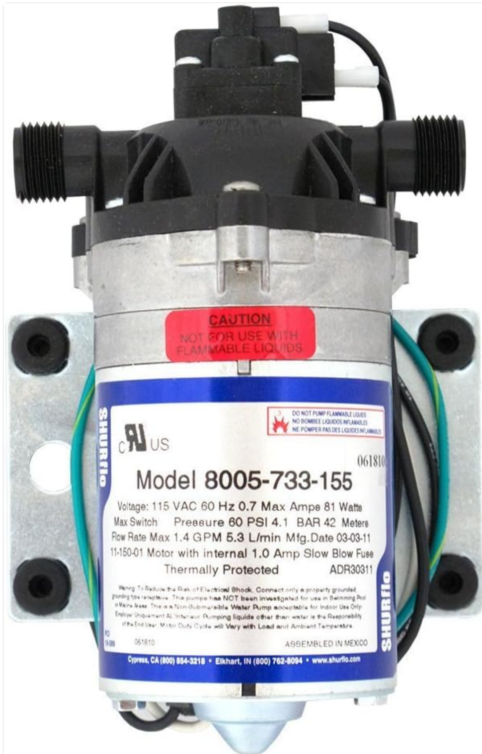
Image: SHURFLO 8005-733-155 Diaphragm Pump. Note the red caution label indicating "NOT FOR USE WITH FLAMMABLE LIQUIDS" and the blue label with model number and electrical specifications.
