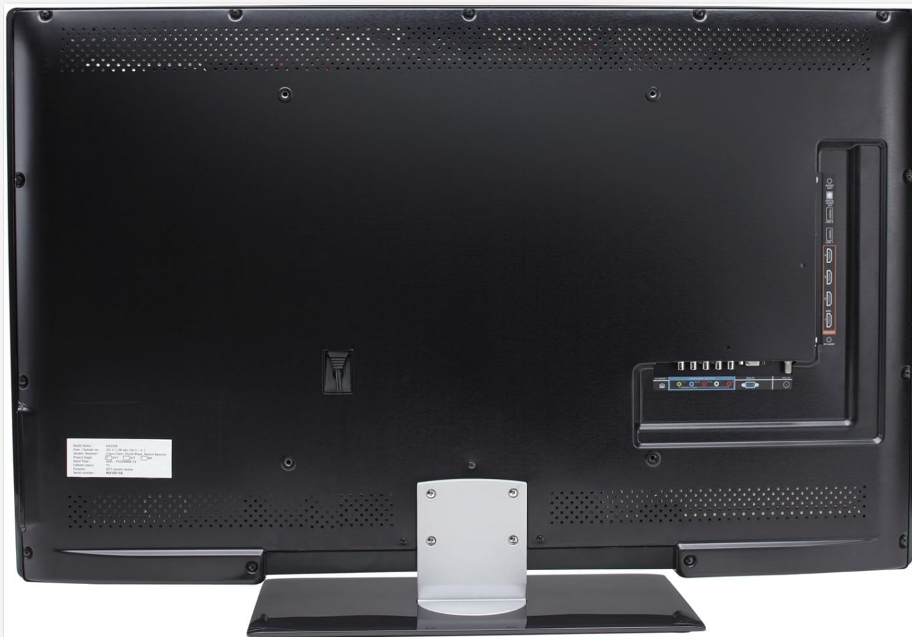
Image: Rear view of the VIZIO M3D420SR TV, highlighting the arrangement of HDMI, USB, and other connectivity ports on the back panel.
