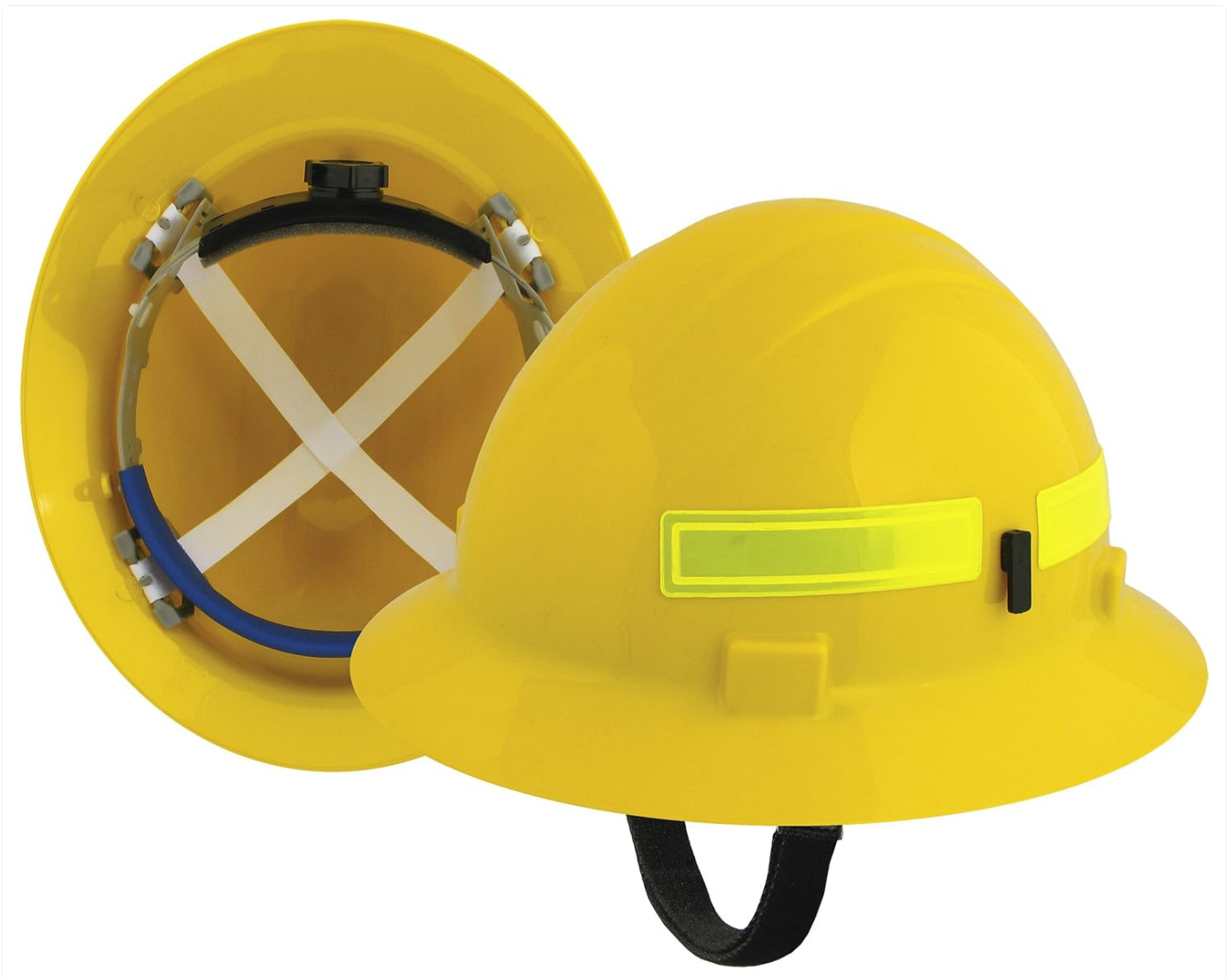
Figure 1: The ERB 19752 Americana Wildlands Full Brim Hard Hat. This image shows the exterior of the yellow hard hat with its full brim and reflective strips, alongside an inverted view revealing the internal 4-point woven nylon suspension system and the Mega Ratchet adjustment mechanism.
