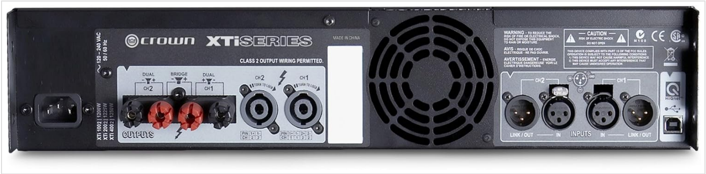
Figure 3.3: Rear panel of the Crown XTi2002 amplifier, showing input (XLR), output (Speakon, Binding Post), and power connections.
