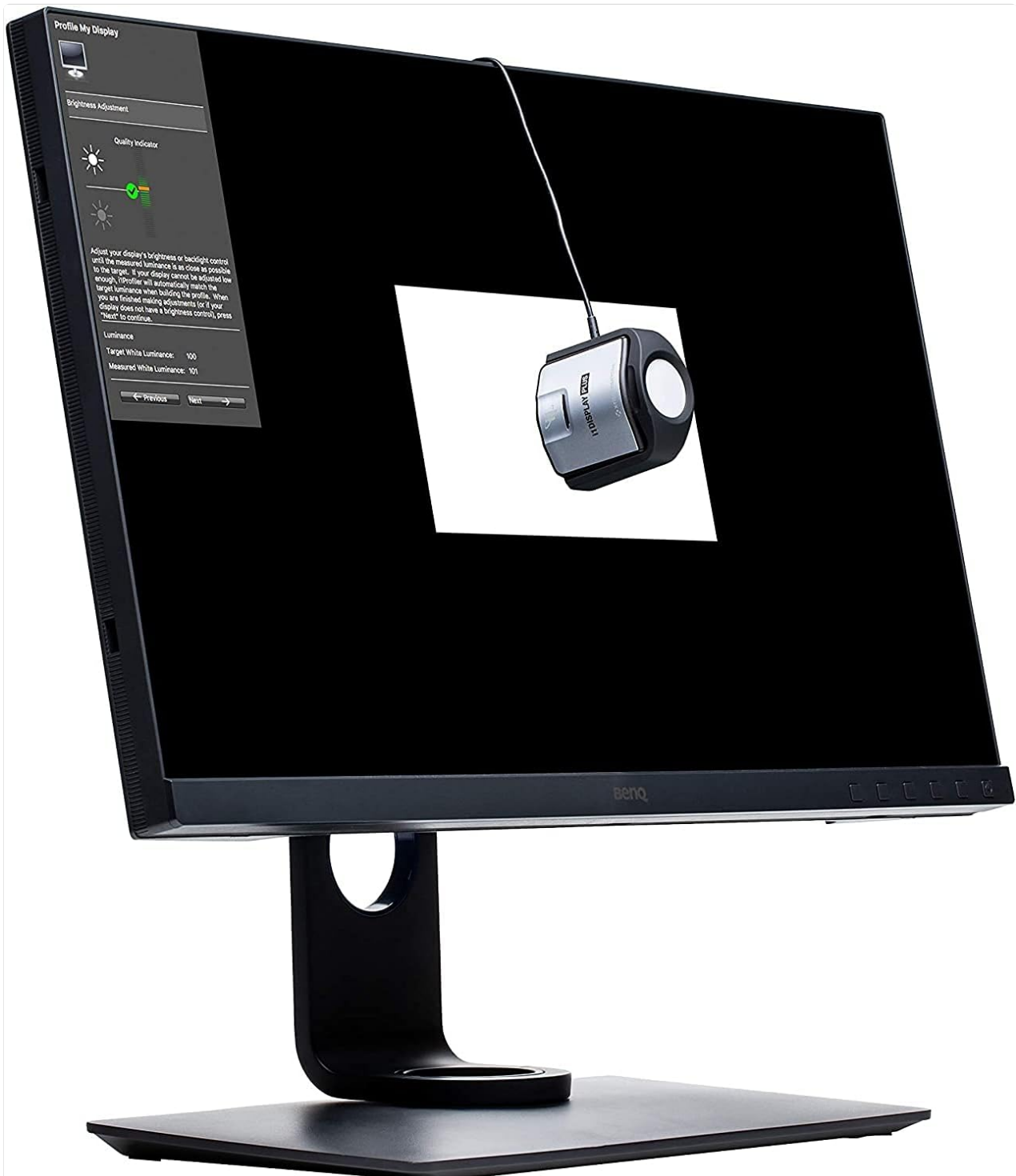
Image 4.1: The i1Display Pro positioned on a monitor for accurate color measurement.
