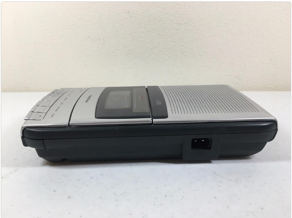
Figure 3: Right side view of the recorder, showing the DC power input jack.
