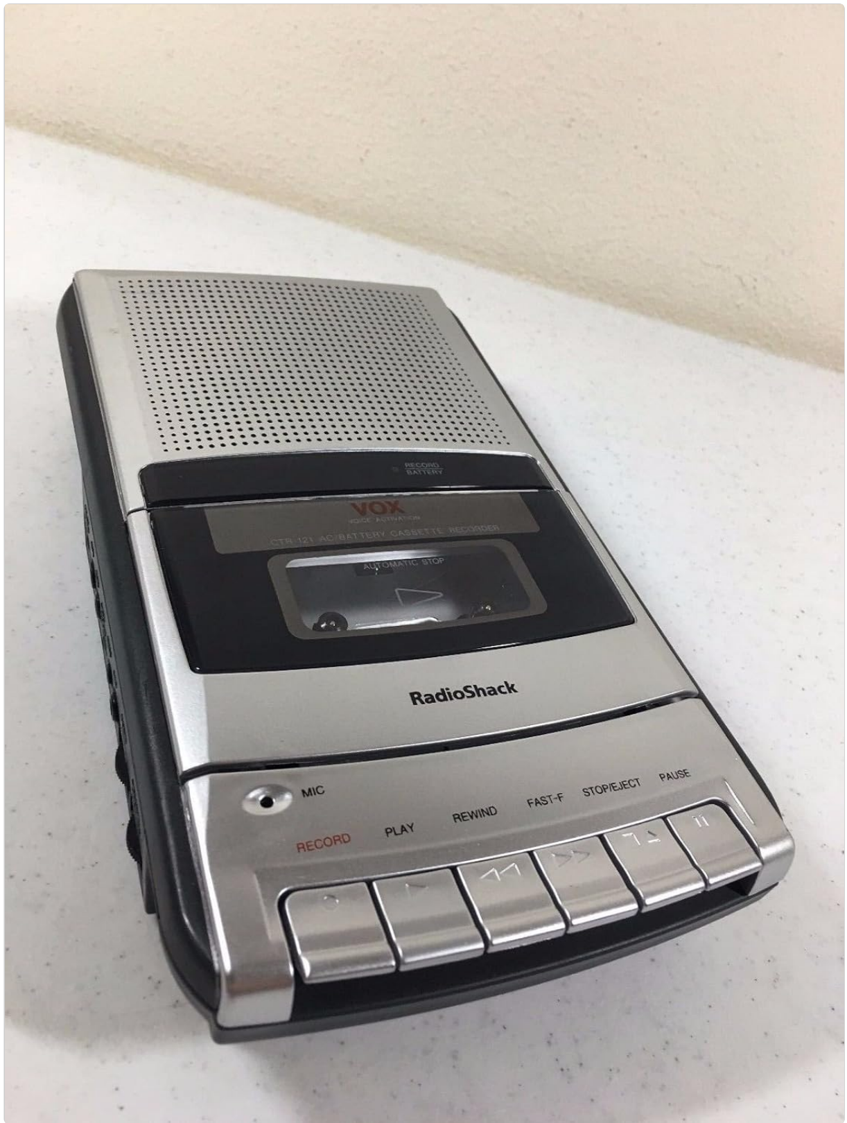
Figure 1: Front view of the RadioShack CTR-121 Desktop Cassette Recorder, showing the speaker, cassette compartment, and control buttons.
