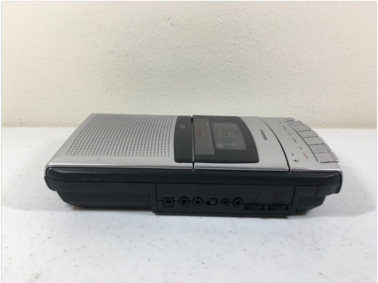
Figure 2: Left side view of the recorder, illustrating the microphone, earphone, and remote control jacks.
