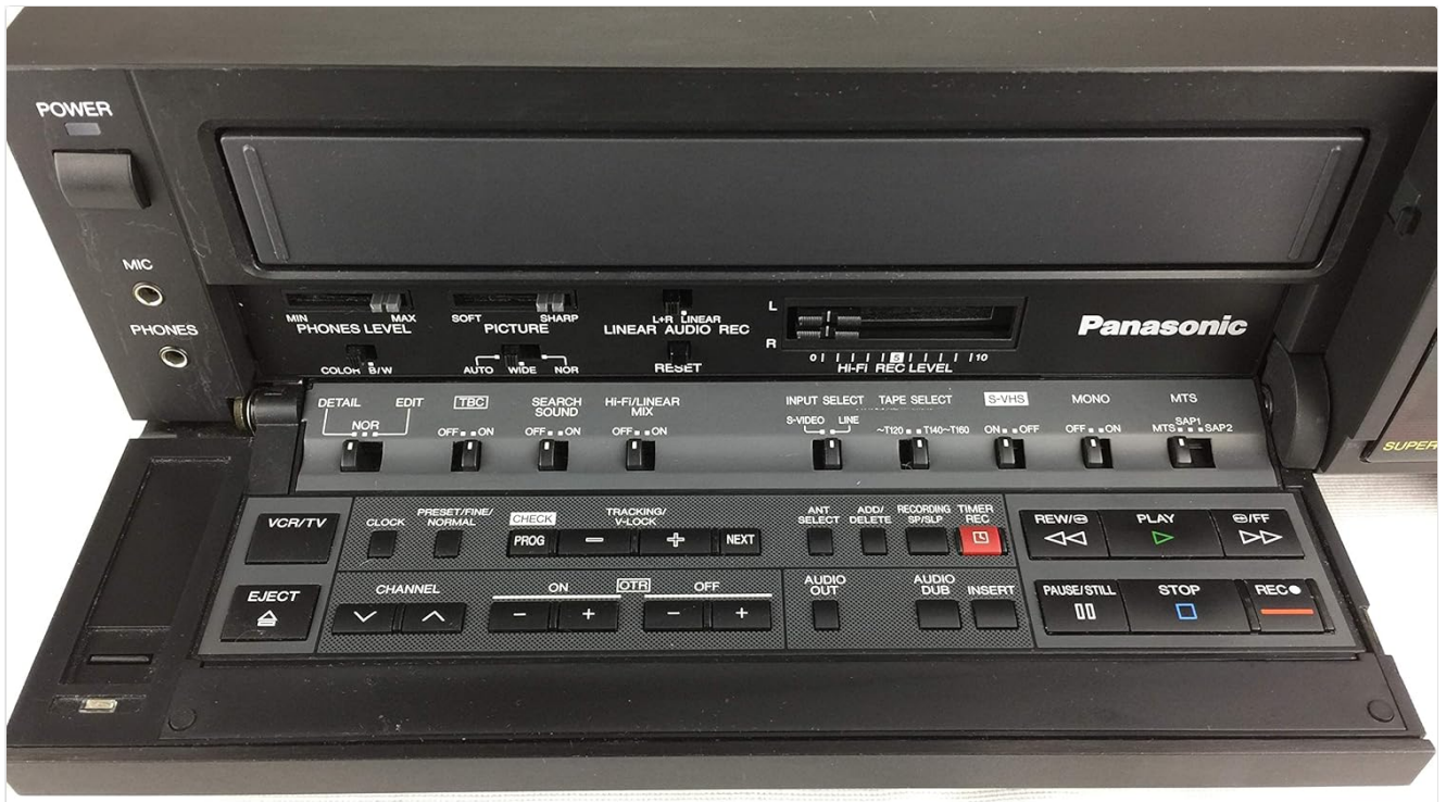
Figure 3: Detailed view of the AG-1980's hidden control panel, highlighting the TBC, DNR, audio level controls, and editing buttons.
