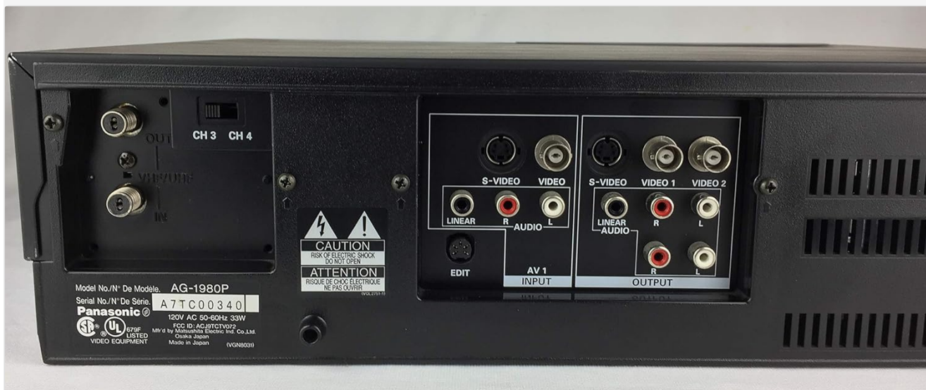
Figure 1: Rear panel connections of the Panasonic AG-1980, illustrating S-Video, BNC, and RCA input/output ports for video and audio, along with the 5-pin editing terminal.
