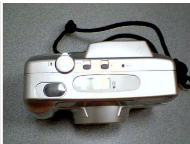
Image: Rear view of the Vivitar PZ3115 camera, displaying the film counter, mode select, and set buttons for the Date-A-Print function.
