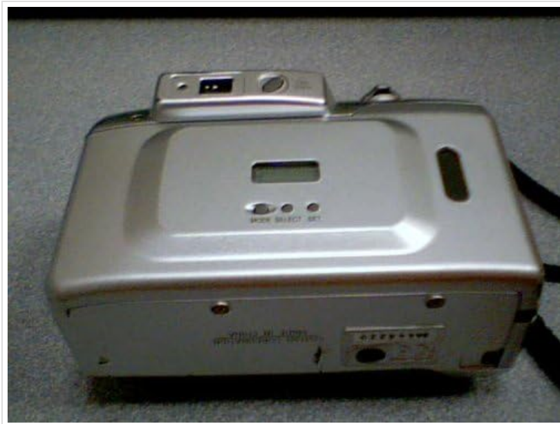
Image: Rear view of the Vivitar PZ3115 camera, displaying the film counter, mode select, and set buttons for the Date-A-Print function.
