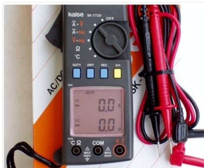
Figure 2: Detailed view of the SK-7722's dual LCD display, rotary function dial, and control buttons.
