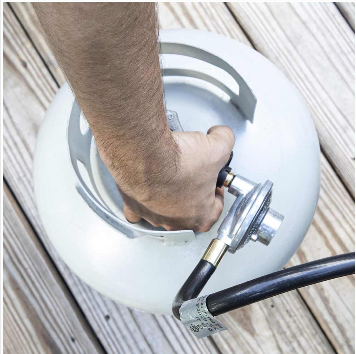
Image 3.2: A hand connecting the regulator hose to a propane tank, illustrating the proper attachment method.
