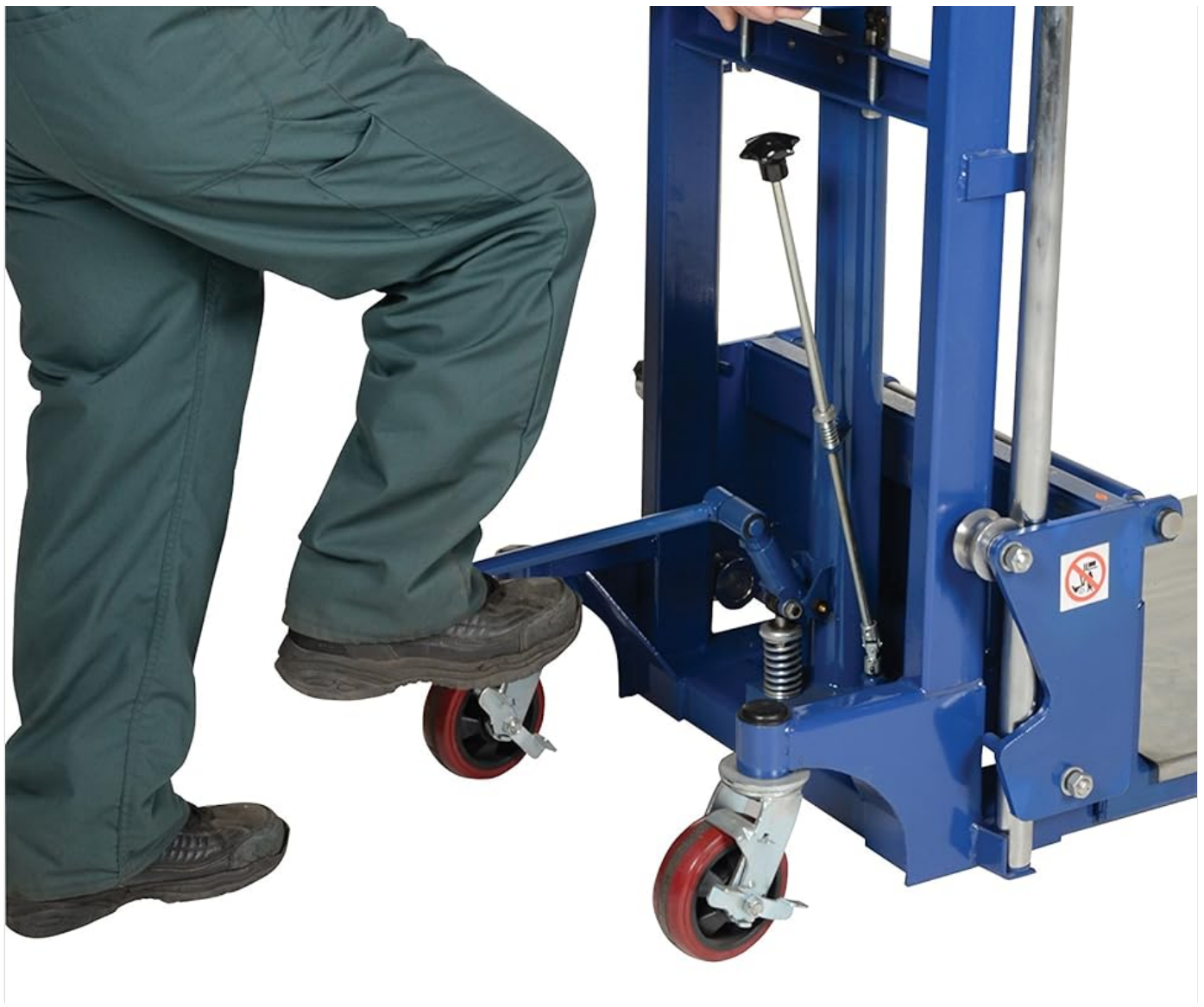
Figure 3: Operating the foot pump to raise the platform.
