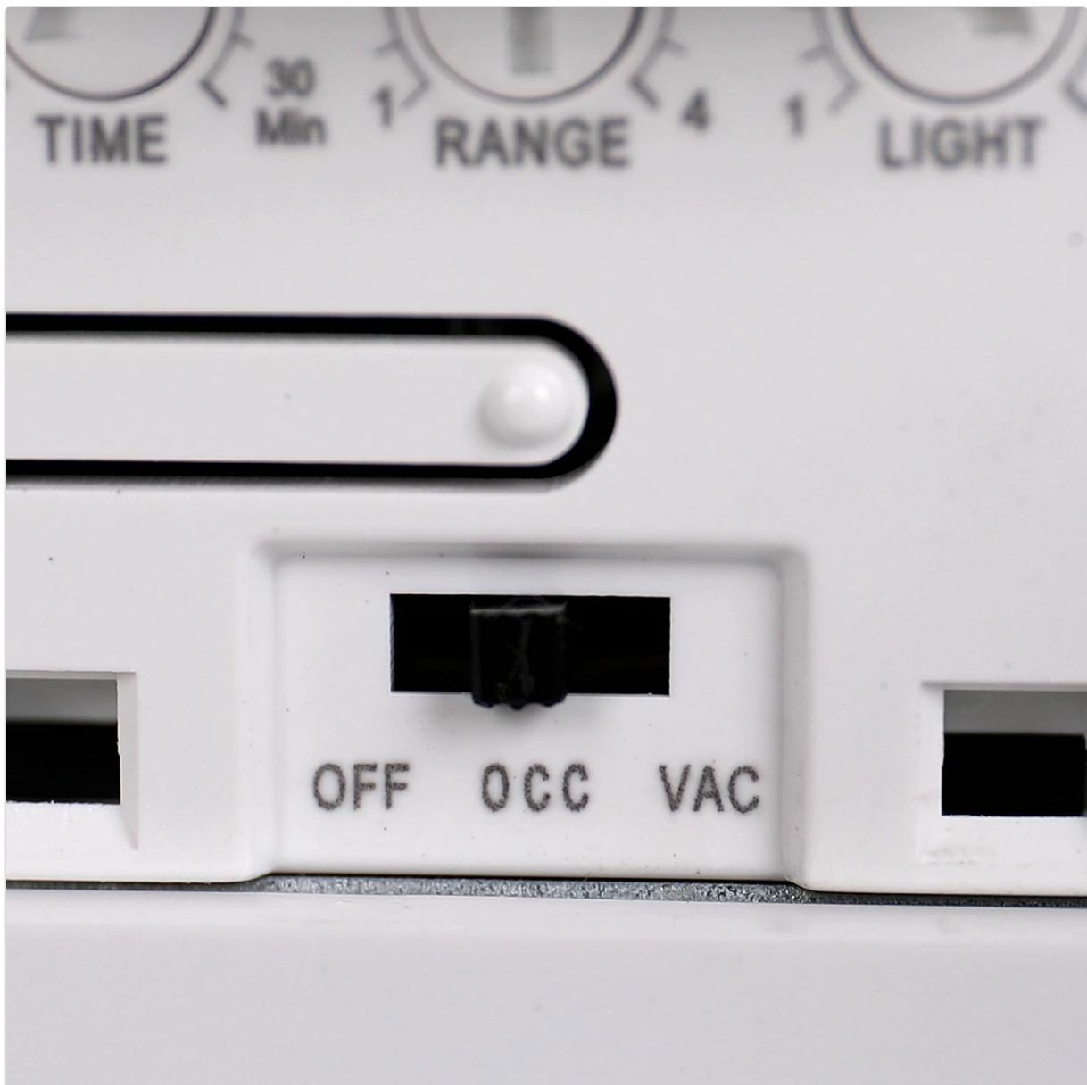
Image 4: A close-up view of the mode selection switch located at the bottom of the sensor. The switch allows selection between "OFF", "OCC" (Occupancy), and "VAC" (Vacancy) modes.
