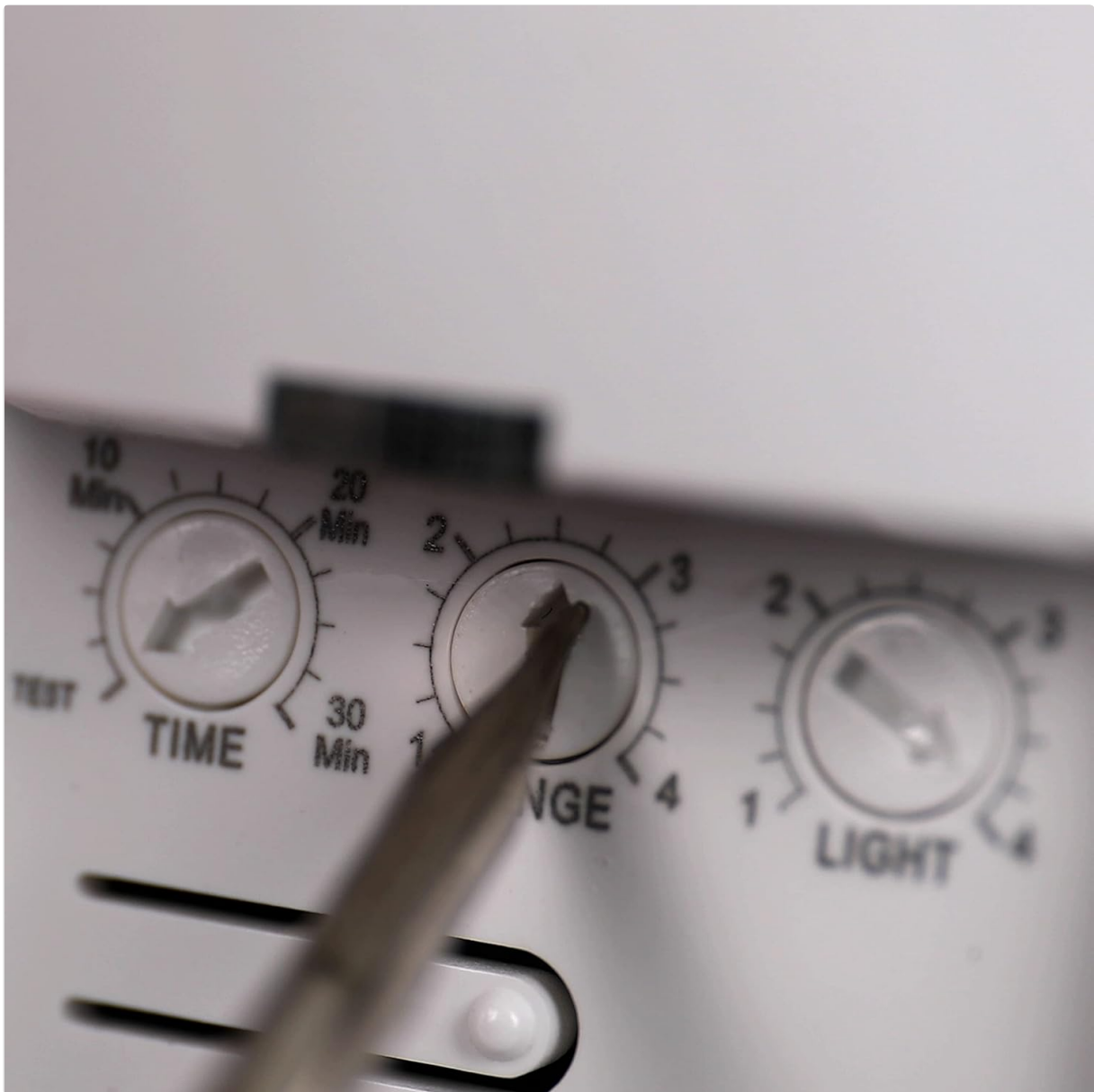
Image 7: This image illustrates the use of a small screwdriver to adjust the "RANGE" dial on the Intermatic iOS-DOV-WH sensor, providing a visual guide for users making adjustments.
