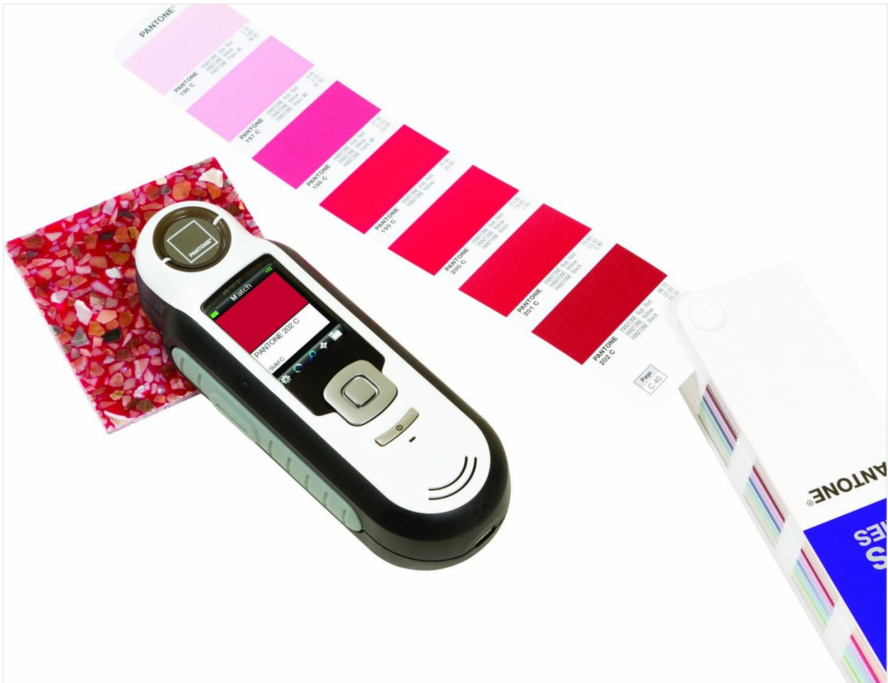
Image: The Pantone Capsure device actively scanning a red textured material, displaying a matched Pantone color on its screen. A Pantone Formula Guide with various red color swatches is visible in the background, illustrating the color matching process.
