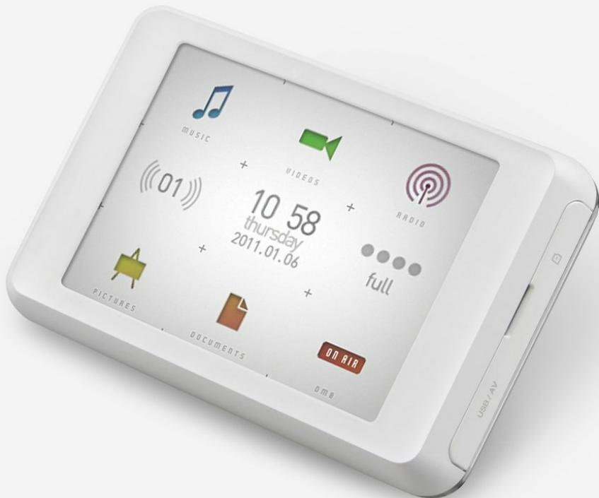
**Figure 1:** Front view of the Cowon C2 Portable Media Player. The screen displays icons for Music, Videos, Radio, Pictures, and Documents. It also shows the current time (10:58), date (Thursday, 2011.01.06), and battery status. A USB/AV port is visible on the side.
