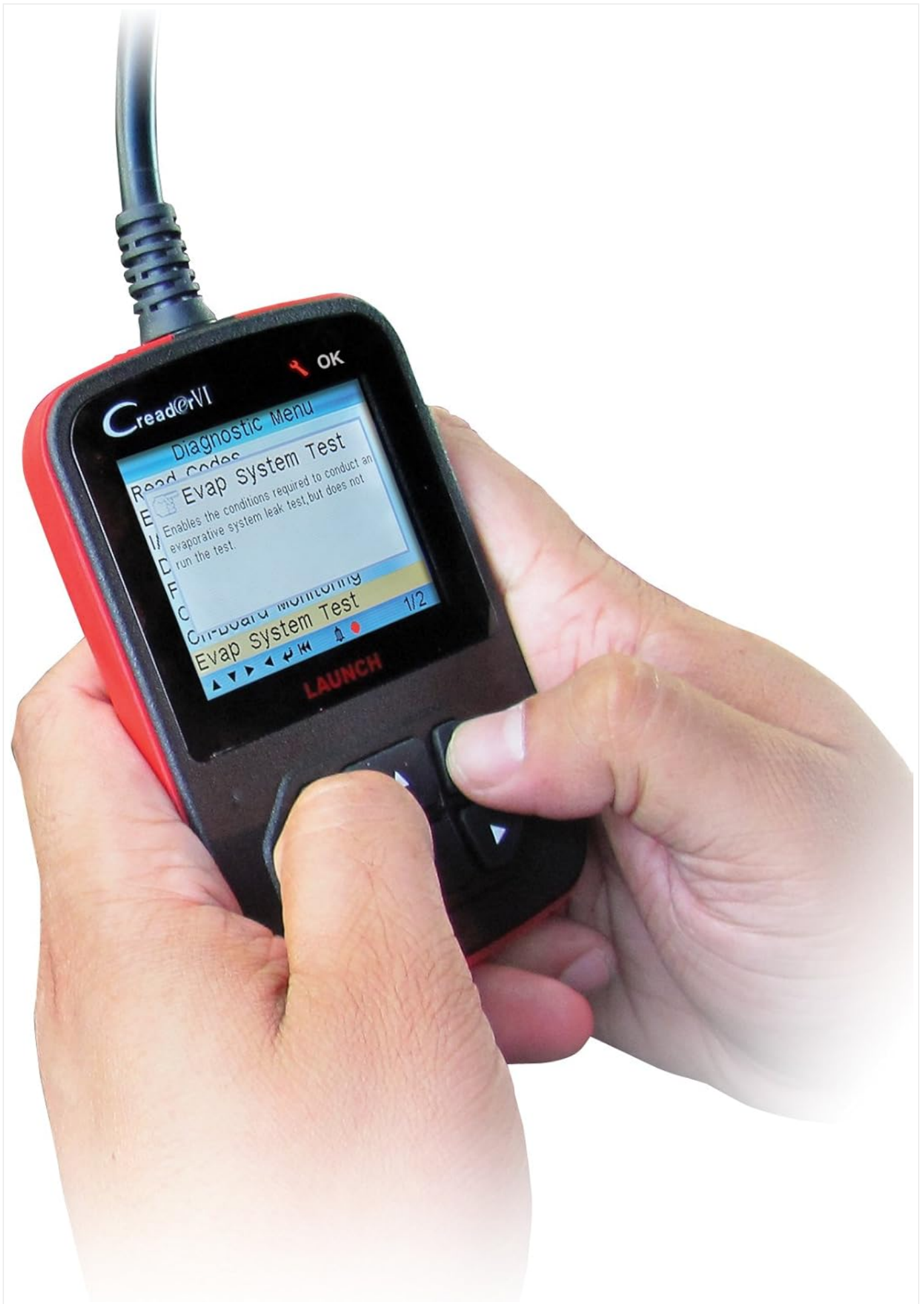
Image: A user's hands operating the Creader VI, displaying the 'Diagnostic Menu' with various test options.
