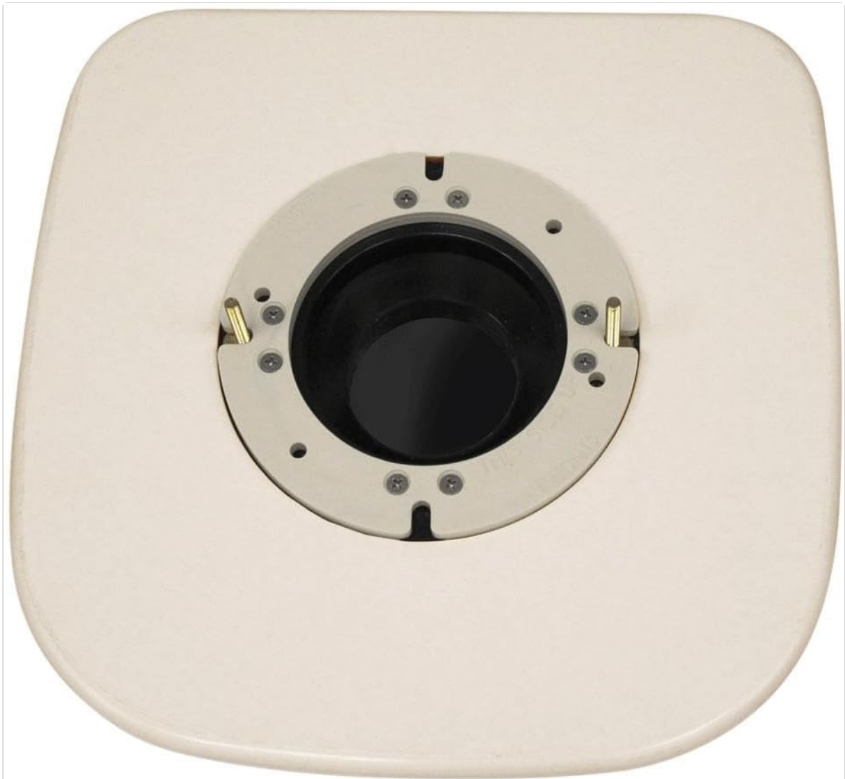
Figure 1: Top view of the Dometic Toilet Mounting Adapter Kit. This image shows the adapter plate with the central opening for the waste pipe and the various screw holes for securing it to the floor and for attaching the new toilet. The two brass-colored pins indicate the two-bolt mounting points for the new toilet, while the surrounding holes accommodate the original four-bolt pattern.
