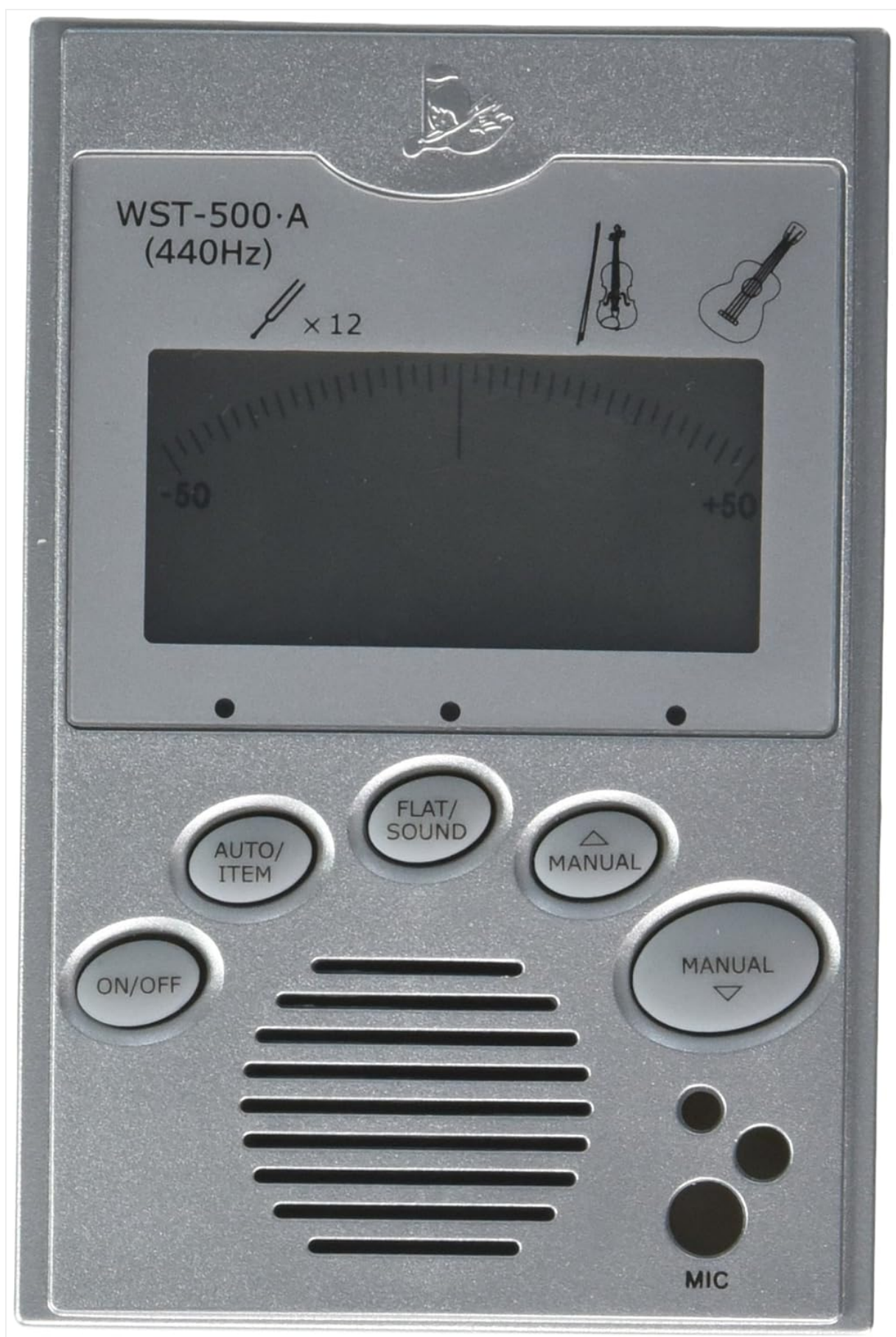
Figure 1: Front view of the Cherub WST-500A Chromatic Tuner, showing the display, control buttons, speaker, and microphone.
