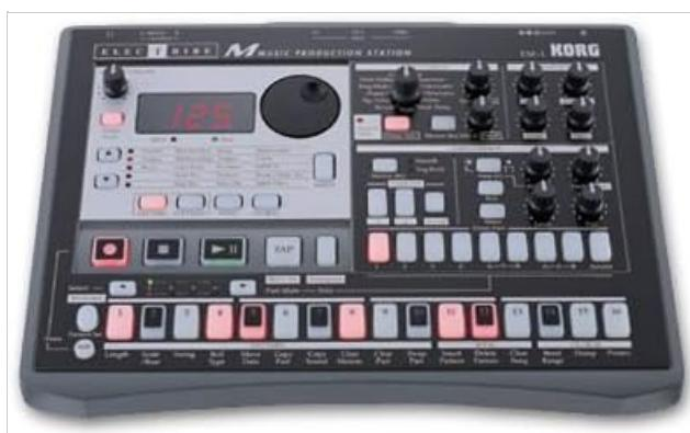
This image displays the Korg Electribe EM-1, highlighting its central LCD screen, various rotary encoders for parameter control, illuminated step buttons for sequencing, and dedicated buttons for mode selection and transport. The layout is designed for intuitive workflow in music production.
