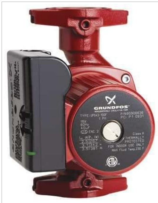
Figure 1: GRUNDFOS UPS43-100F Circulator Pump. This image displays the red cast iron body of the pump with a black electrical terminal box on its left side. The circular nameplate on the front of the pump clearly indicates the model type UPS43-100F, part number P/N 95906636, 1 PH, 115V, 60Hz, and ETL certification. It also specifies that the pump is for indoor use only and has a maximum fluid temperature of 230°F.
