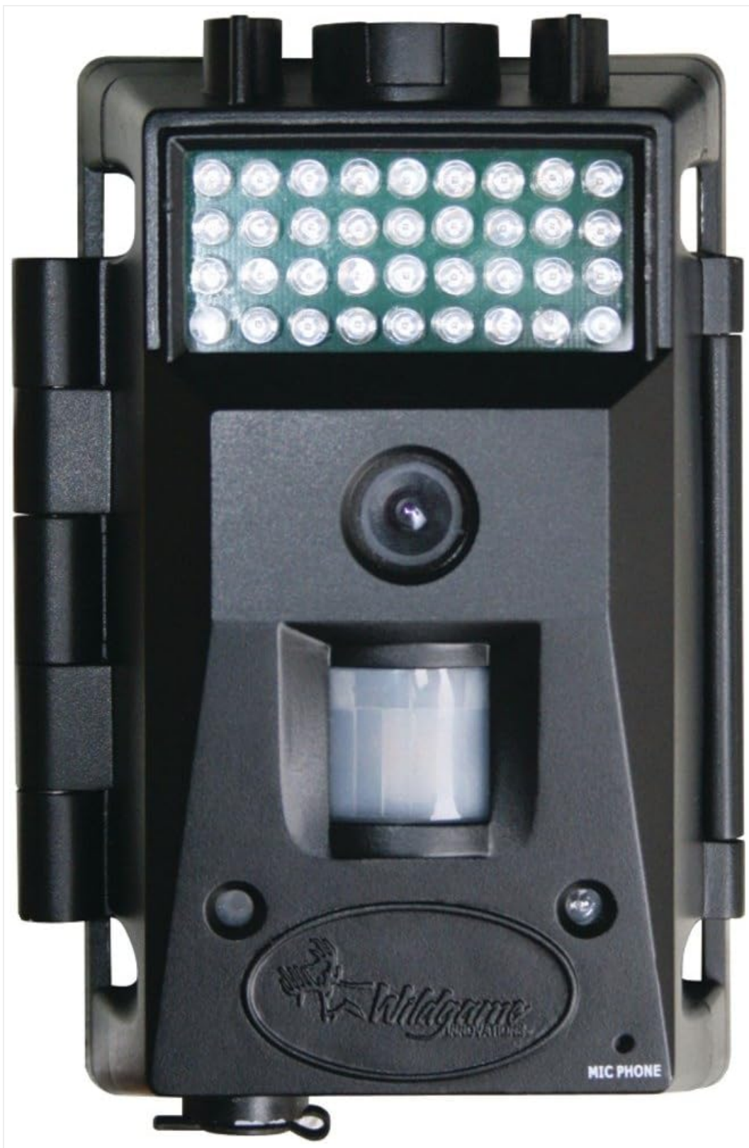
Front view of the Wildgame Innovations Pulse 10 Infrared Digital Scouting Camera, showing the infrared LED array, camera lens, and PIR motion sensor.
