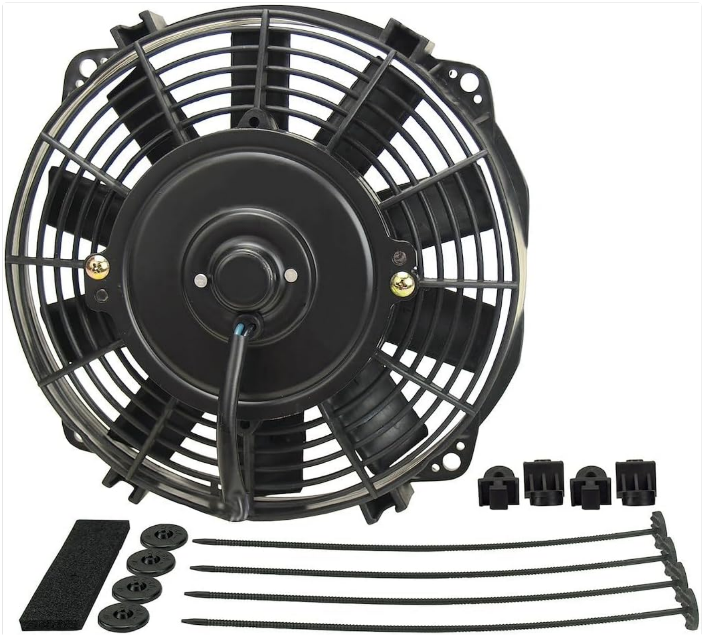
Figure 1: Derale 16908 8" Dyno-Cool Electric Fan with included mounting hardware. The image shows the fan assembly, four plastic through-radiator core rods with clips, four foam pads, and four mounting feet.
