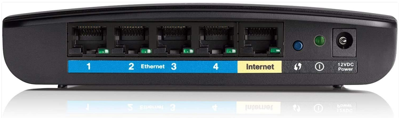
Figure 2: Rear panel of the Linksys E1200 router, highlighting the four blue Ethernet LAN ports (1-4), the yellow Internet WAN port, and the 12VDC Power input.
